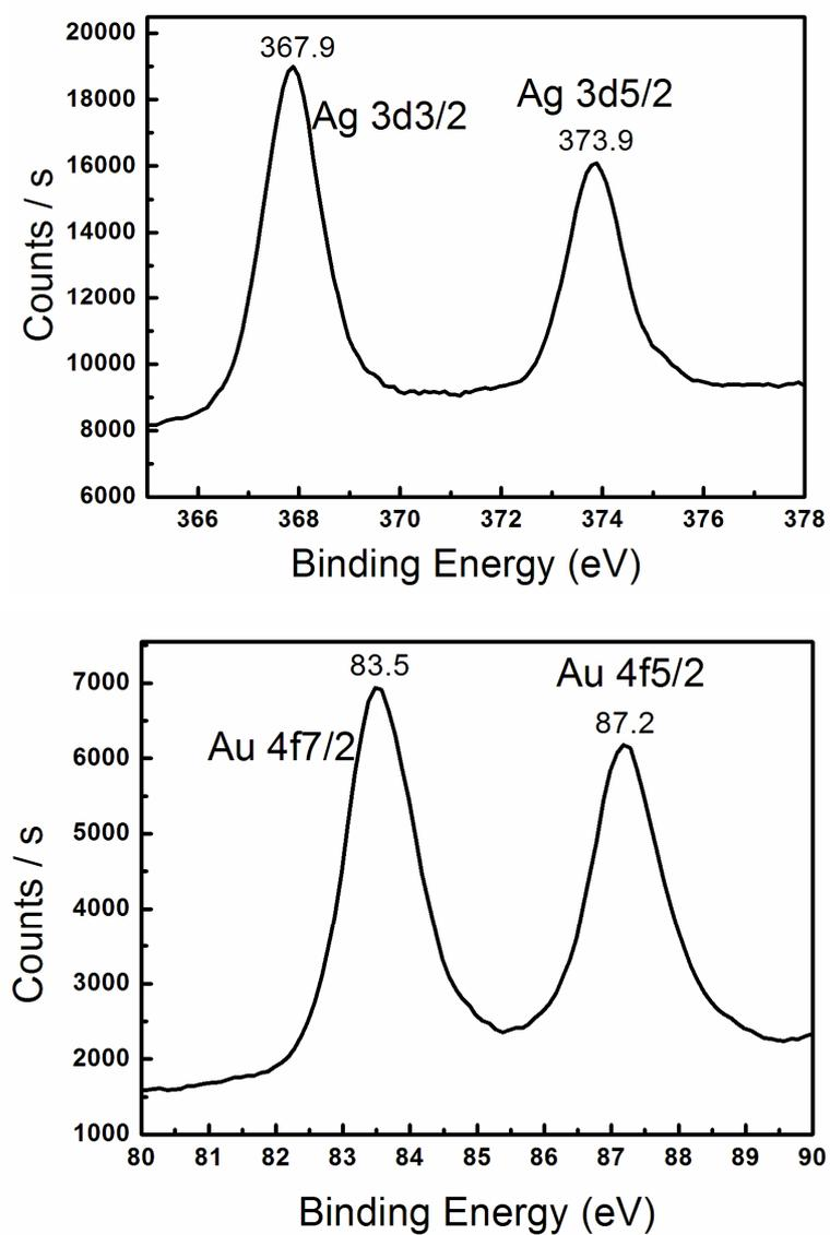
**Fig. S6** High resolution XPS spectra of Ag 3d (a) and Au 4f (b) of the Ag-Au-C composites after being used three times as a catalyst reducing 4-NP.
