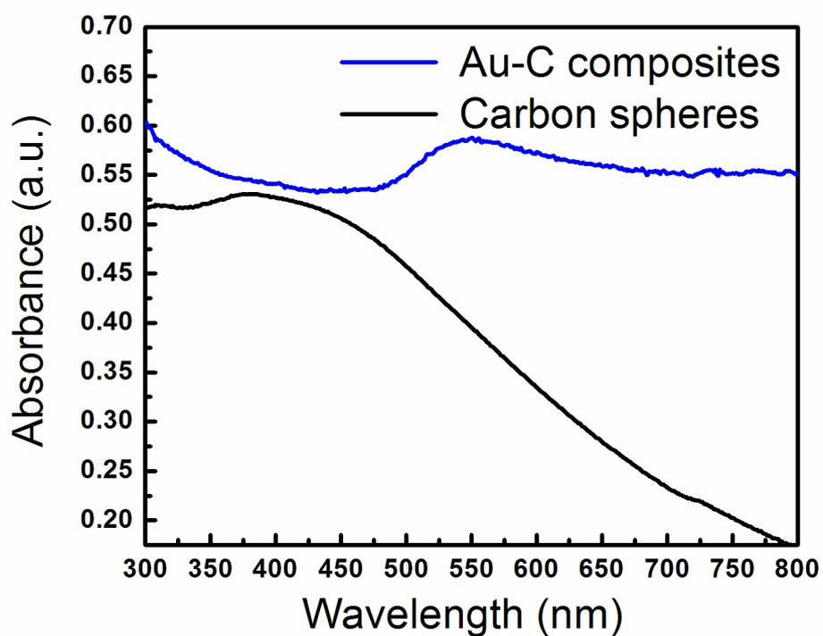
**Fig. S3** UV-Vis absorption spectra of suspension of bare CSs in aqueous solution (black curve) and the product form a microwave synthesis at 140 W for 10 min *without* PVP and even without microwaving (blue curve).
