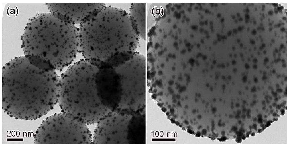
**Fig. S2** TEM images of a product obtained after microwaving a suspension of CSs in  $\text{HAuCl}_4$  solutions ( $C_{\text{HAuCl}_4} = 2 \times 10^{-4} \text{ mol/L}$ ,  $t_I = 4 \text{ h}$ , and MW power  $\langle P \rangle = 140 \text{ W}$ ) in the presence of PVP. Au NPs only formed on the surfaces of the CSs under these conditions (without previous Ag doping).
