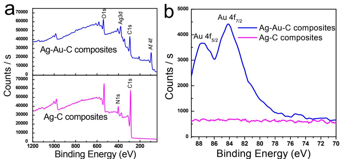
**Fig. S5** XPS survey spectra (a) and XPS Au 4f signals (b) of Ag-C (red line) and Ag-Au-C (blue line) composite particles shown in Fig. 1b and 5a.
