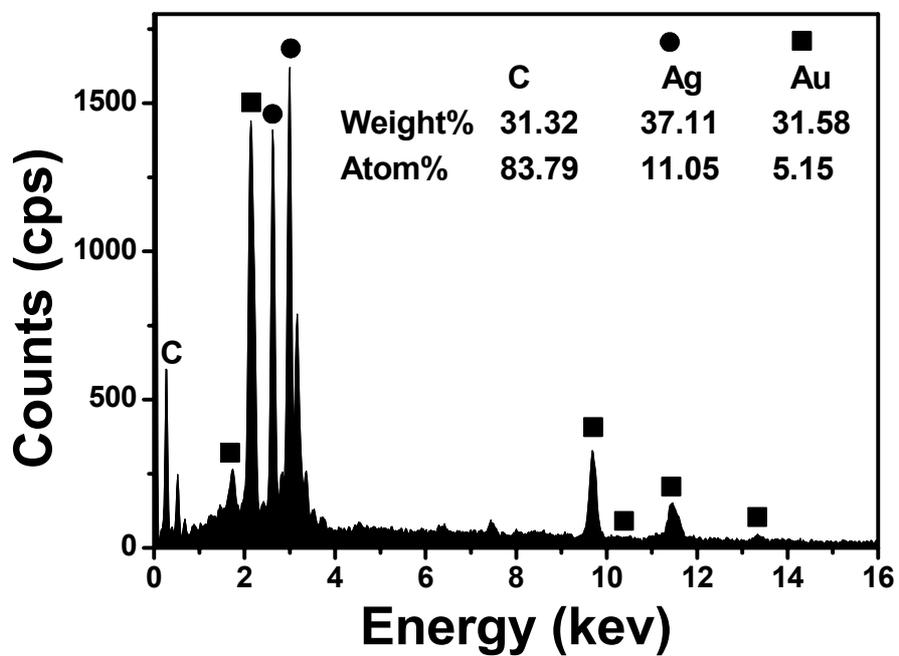
**Fig. S4** SEM-EDS spectrum recorded from the product shown in Fig. 6e.
