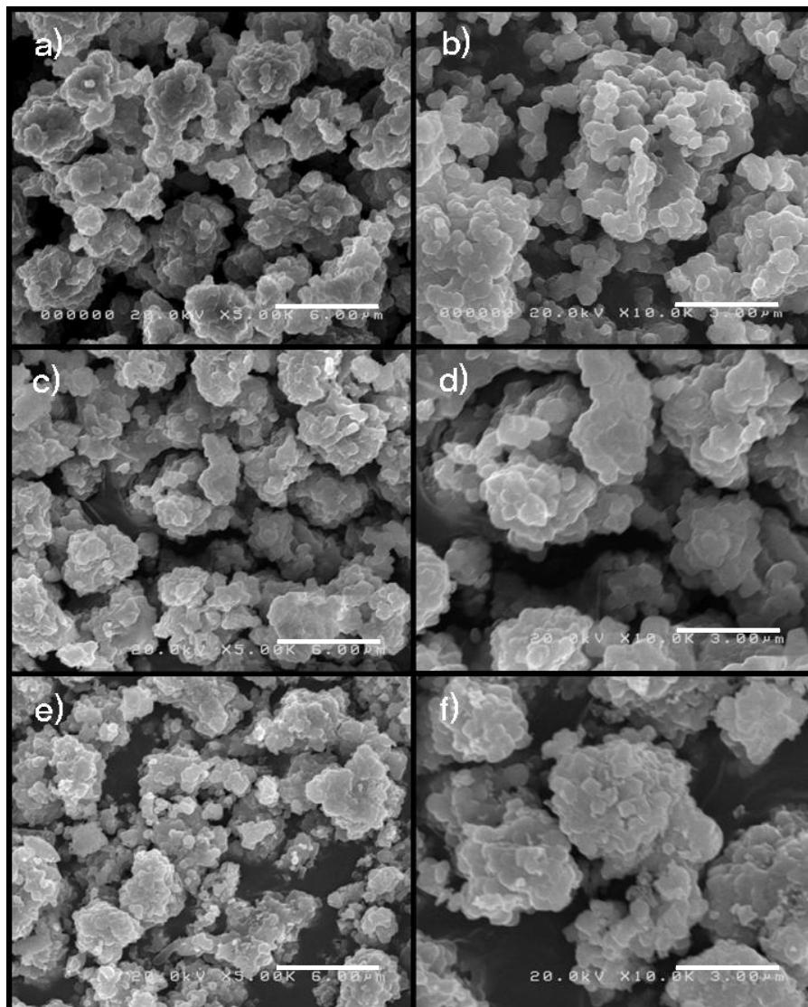
**Fig. S1** FESEM images of (a) and (b) the pristine LNCMM, (c) and (d) the  $\text{Al}_2\text{O}_3$  modified LNCMM, (e) and (f) the  $\text{AlPO}_4$  modified LNCMM at different magnifications.
