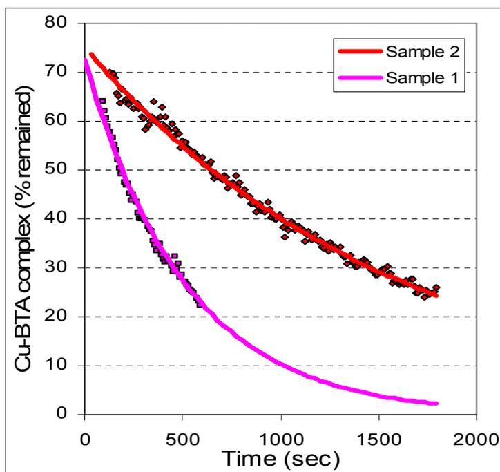
**Fig.1.** Decomposition kinetics of Cu-BTA complex by ammonia solution: sample #1 and sample #2 (with 0.5 % iron).
