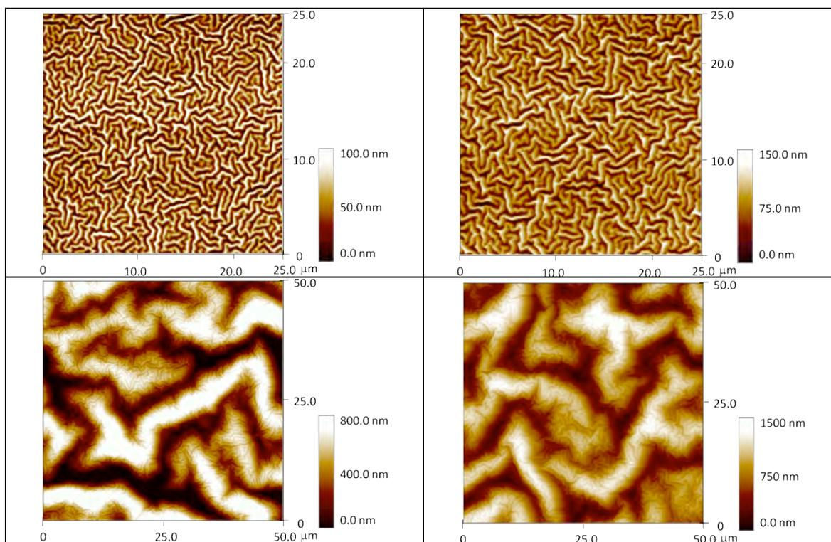
Figure 11S: AFM micrographs of chromium-coated PDMS samples. A: 5 nm chromium coating. B: 15 nm chromium coating. C: 30 nm chromium coating. D: 50 nm chromium coating.
