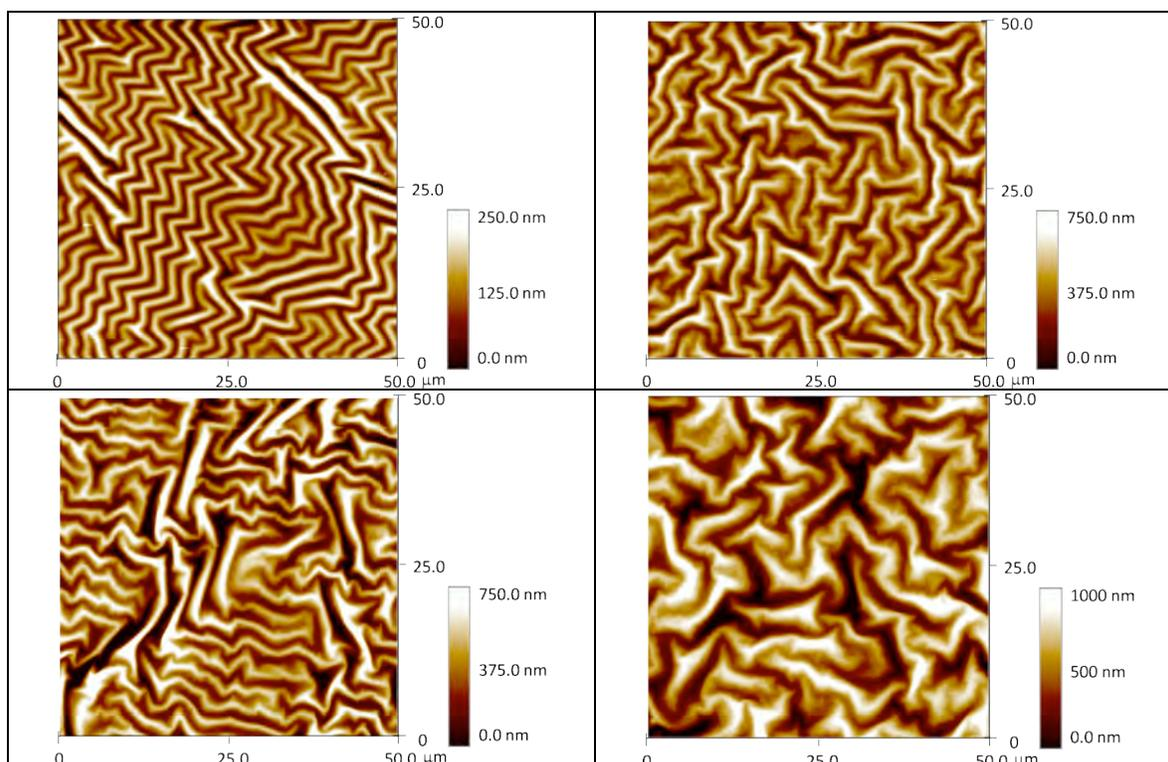
Figure 9S: AFM micrographs of tungsten-coated PDMS samples. A: 5 nm tungsten coating. B: 15 nm tungsten coating. C: 30 nm tungsten coating. D: 50 nm tungsten coating.
