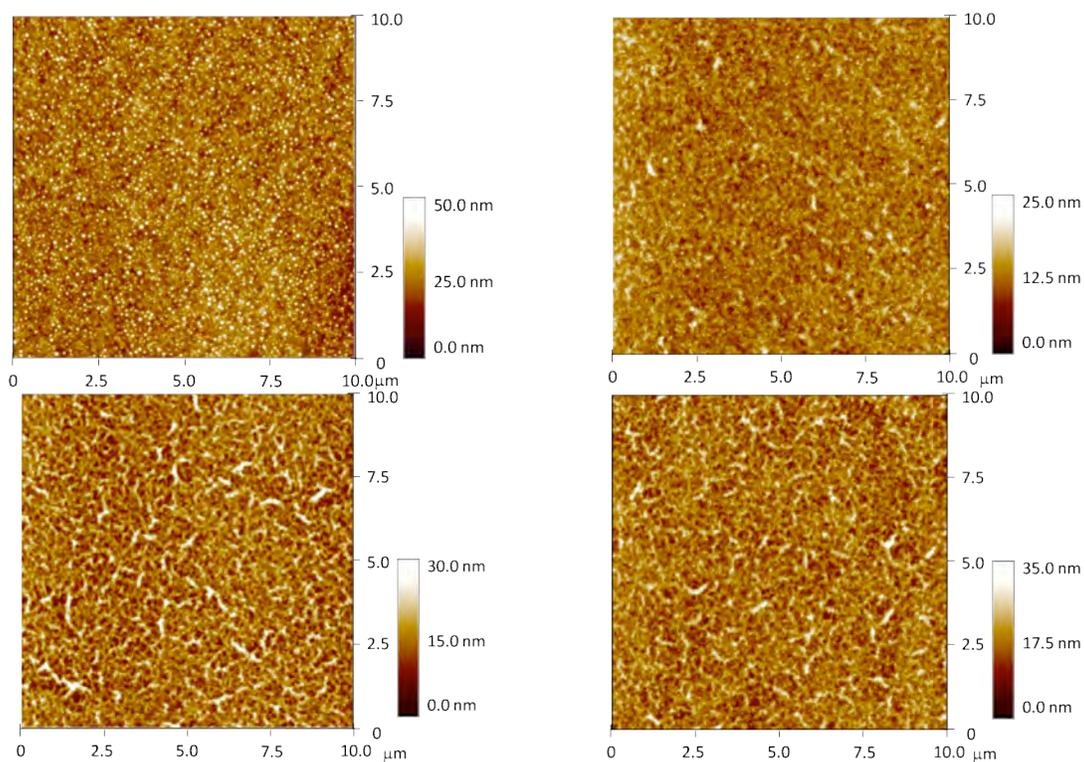
Figure S5: AFM micrographs of gold-coated PDMS samples. A: 5 nm gold coating. B: 15 nm gold coating. C: 30 nm gold coating. D: 50 nm gold coating.
