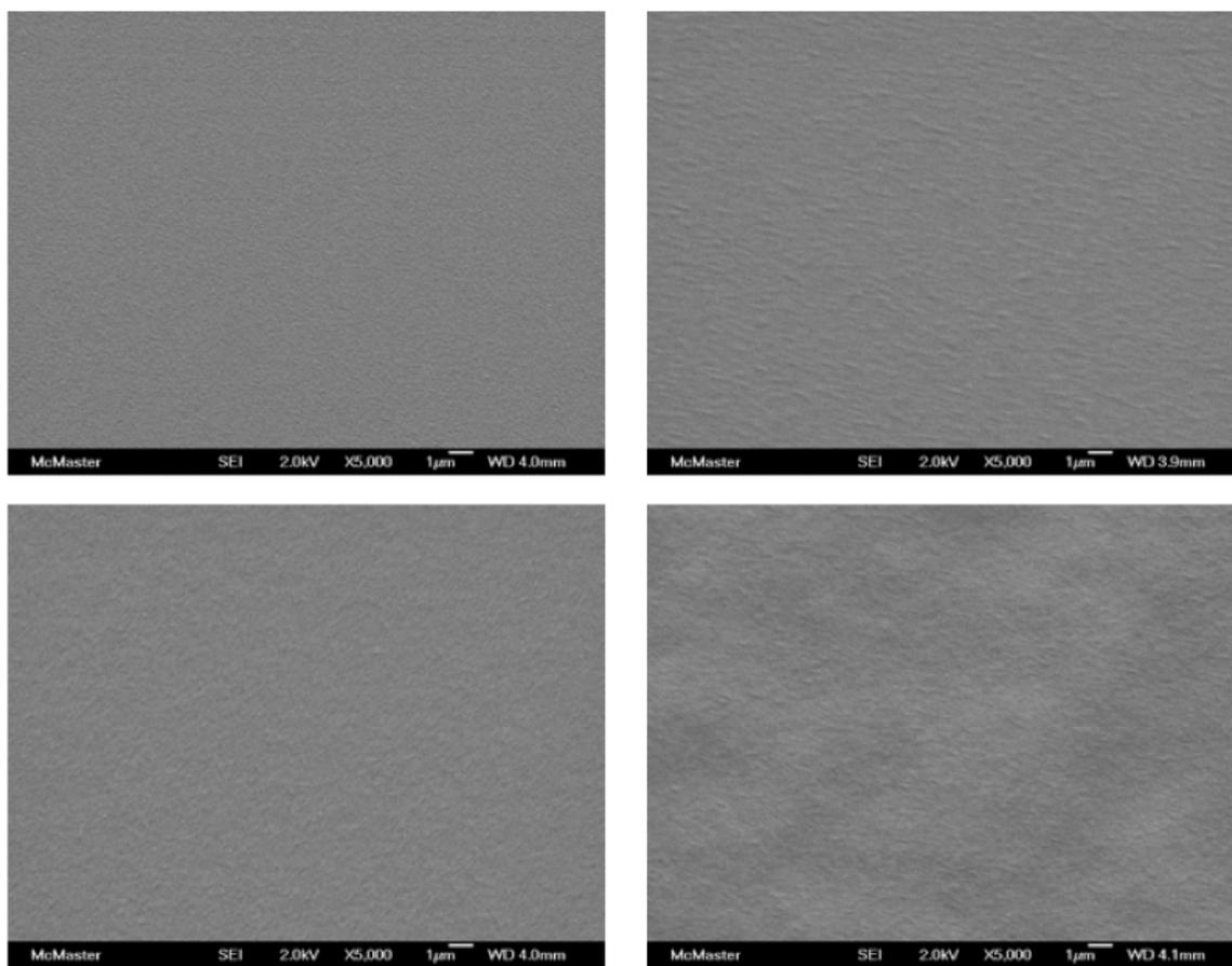
Figure 4S: SEM micrographs of gold-coated PDMS samples. A: 5 nm gold coating. B: 15 nm gold coating. C: 30 nm gold coating. D: 50 nm gold coating. Large scale bar is 10 µm.
