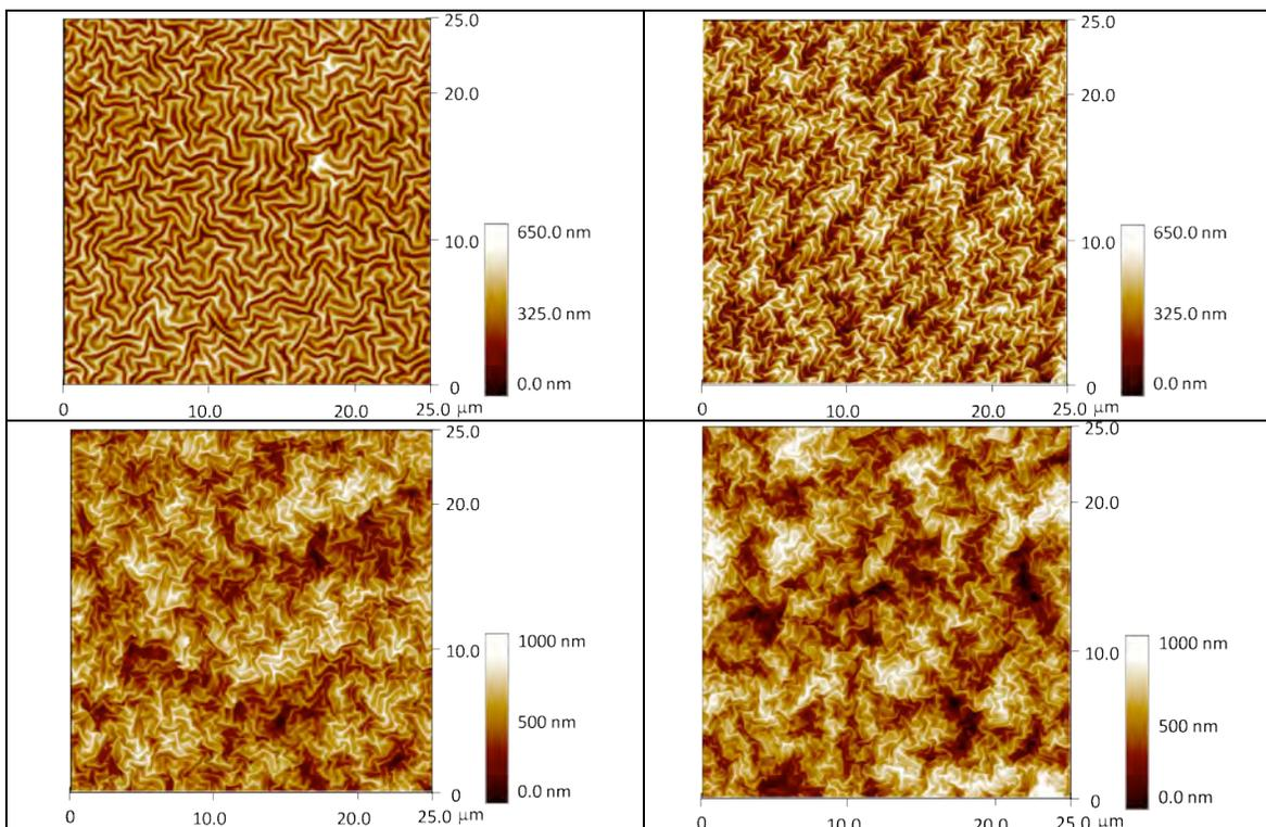
Figure 13S: AFM micrographs of carbon-coated PDMS samples. A: 5 nm carbon coating. B: 15 nm carbon coating. C: 30 nm carbon coating. D: 50 nm carbon coating.
