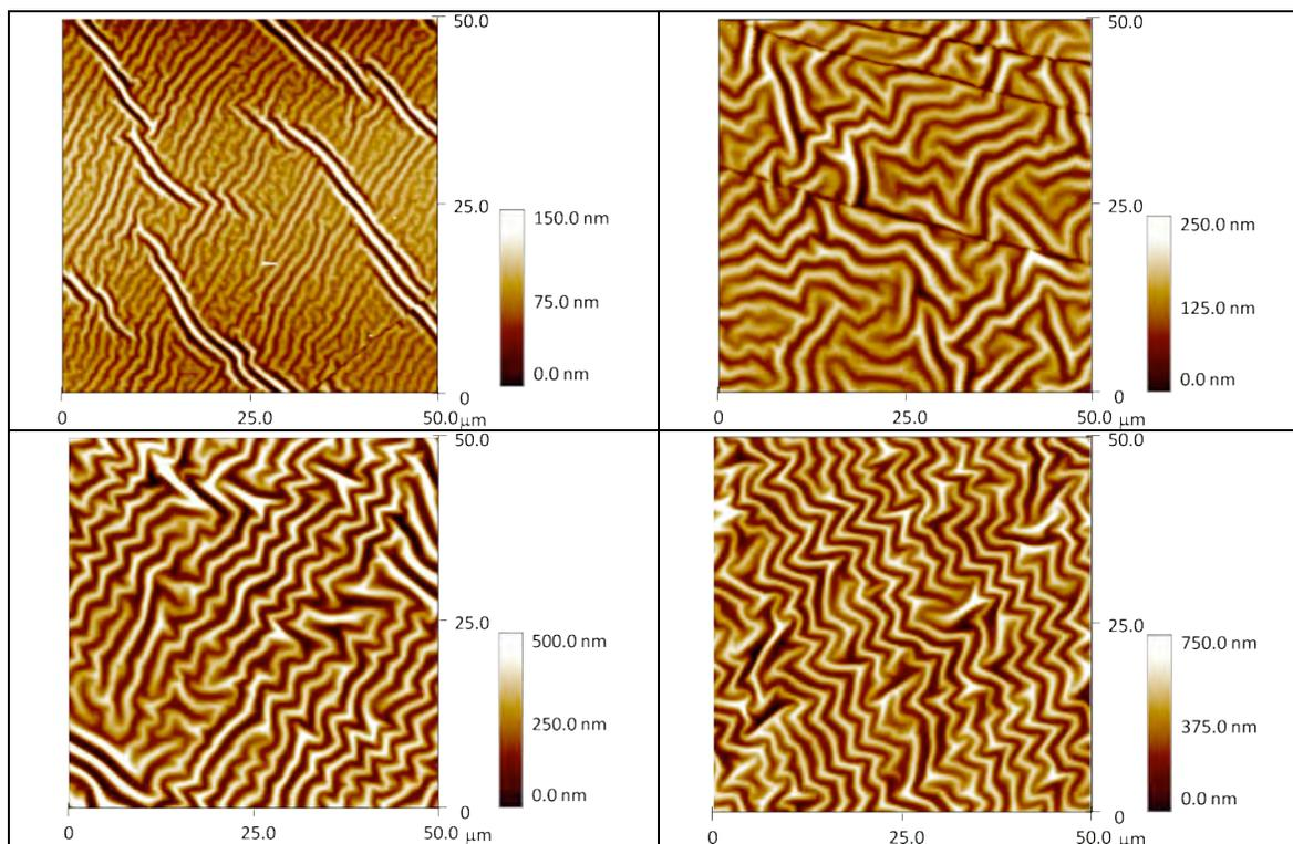
Figure 7S: AFM micrographs of platinum-coated PDMS samples. A: 5 nm platinum coating. B: 15 nm platinum coating. C: 30 nm platinum coating. D: 50 nm platinum coating.
