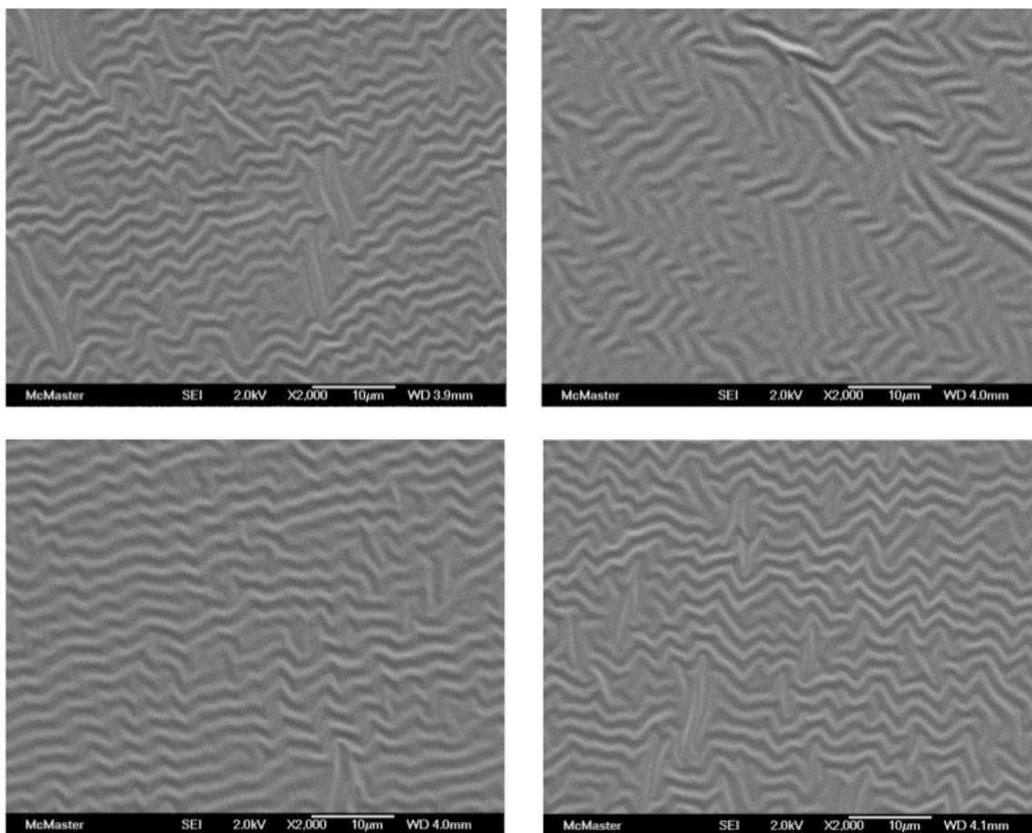
Figure 3S: Comparison of different coating settings: SEM micrographs of 15 nm platinum-coated PDMS samples. A: no rotation, no rocking. B: rocking ( $30^\circ$ ,  $16^\circ/\text{sec}$ ). C: rotation (30 rpm). D: rocking ( $30^\circ$ ,  $16^\circ/\text{sec}$ ) and rotation (30 rpm). The scale bar represents 20  $\mu\text{m}$ .
