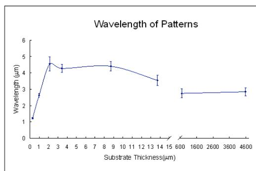
Figure 14S: Comparison of wavelengths of patterns on thin silicone films.
