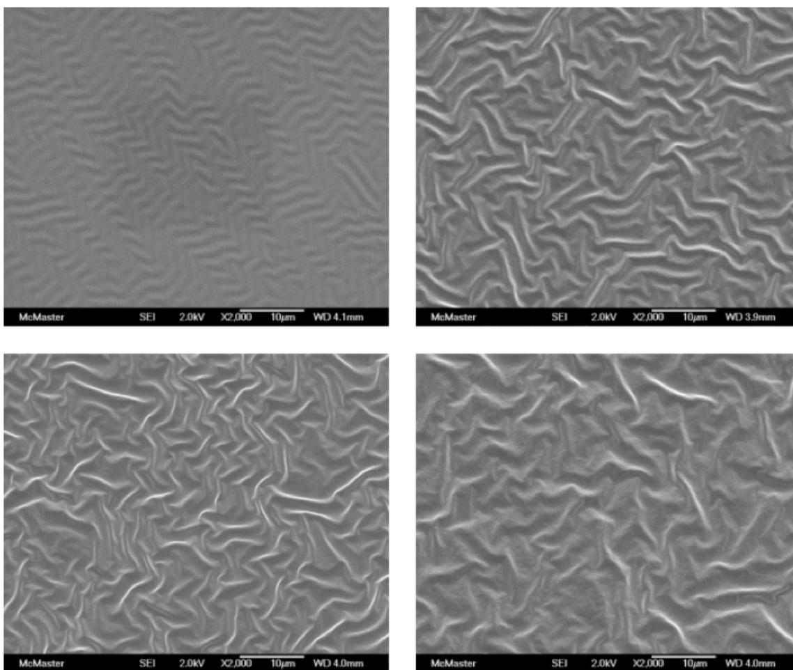
Figure 8S: SEM micrographs of tungsten-coated PDMS samples. A: 5 nm tungsten coating. B: 15 nm tungsten coating. C: 30 nm tungsten coating. D: 50 nm tungsten coating. Scale bar is 10  $\mu\text{m}$ .
