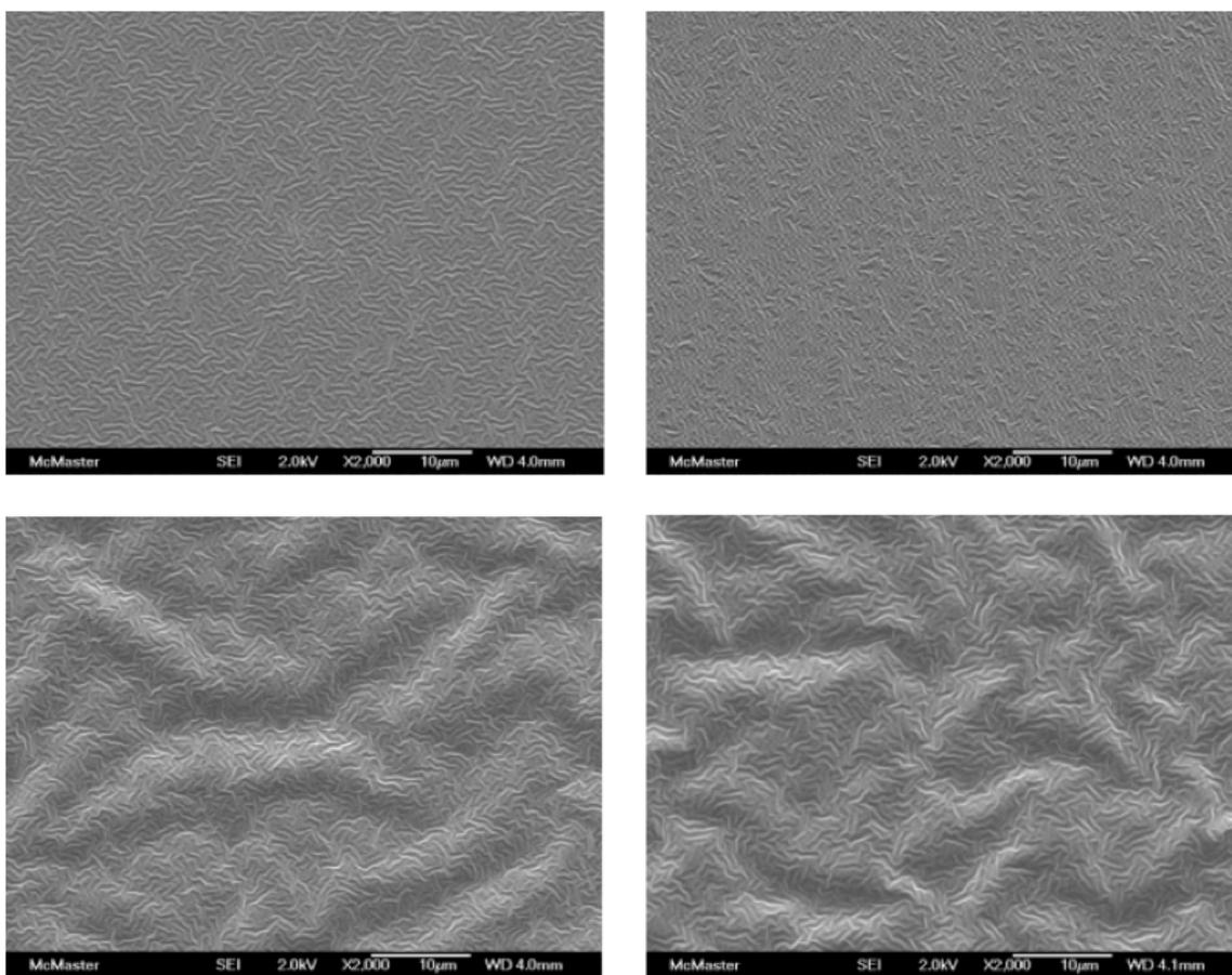
Figure 10S: SEM micrographs of chromium-coated PDMS samples. A: 5 nm chromium coating. B: 15 nm chromium coating. C: 30 nm chromium coating. D: 50 nm chromium coating. Scale bar is 10 μm.
