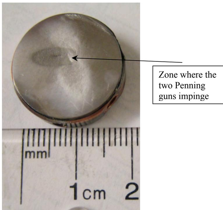
Figure 2S: Metal target (W) showing impingement zone of the Argon ions.
