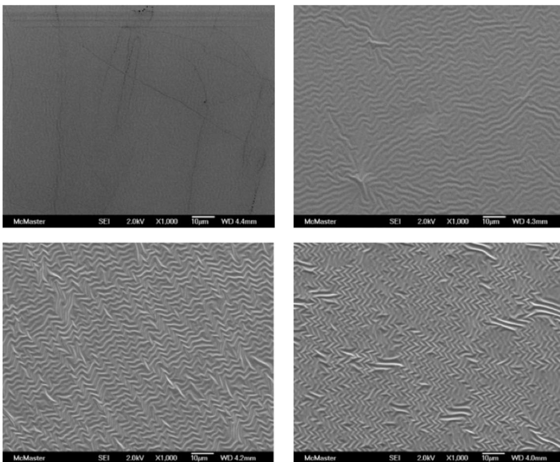
Figure 6S: SEM micrographs of platinum-coated PDMS samples. A: 5 nm platinum coating. B: 15 nm platinum coating. C: 30 nm platinum coating. D: 50 nm platinum coating. Scale bar is 10 μm.
