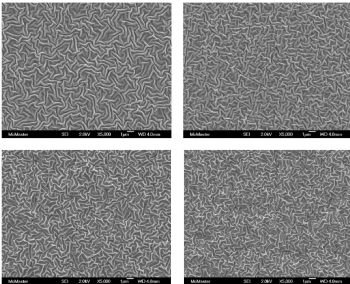
Figure 12S: SEM micrographs of carbon-coated PDMS samples. A: 5 nm carbon coating. B: 15 nm carbon coating. C: 30 nm carbon coating. D: 50 nm carbon coating. Large scalebar is 10  $\mu\text{m}$ .
