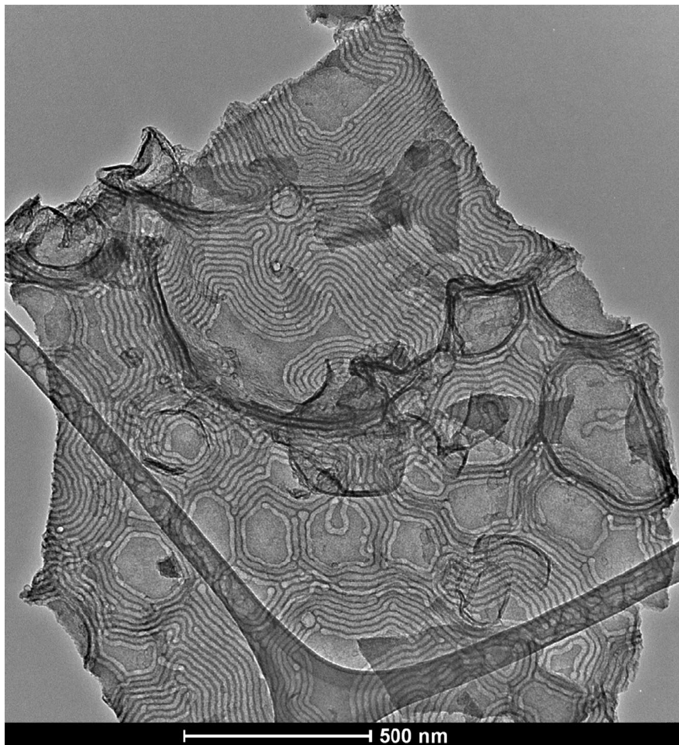
**Supporting Figure S10.** TEM image of extracted ethylene-bridged PMO synthesized at an initial temperature of 11.00 °C.
