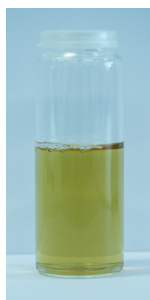
Fig. S2 A yellow appearing dispersion of Ag/SiO 2 nanoparticles in water was made by adding 1 mg particles to 10 g water with 0.1 wt% Disperbyk-190 (BYK-Chemie GmbH) and ultrasonification for 5 minutes.
