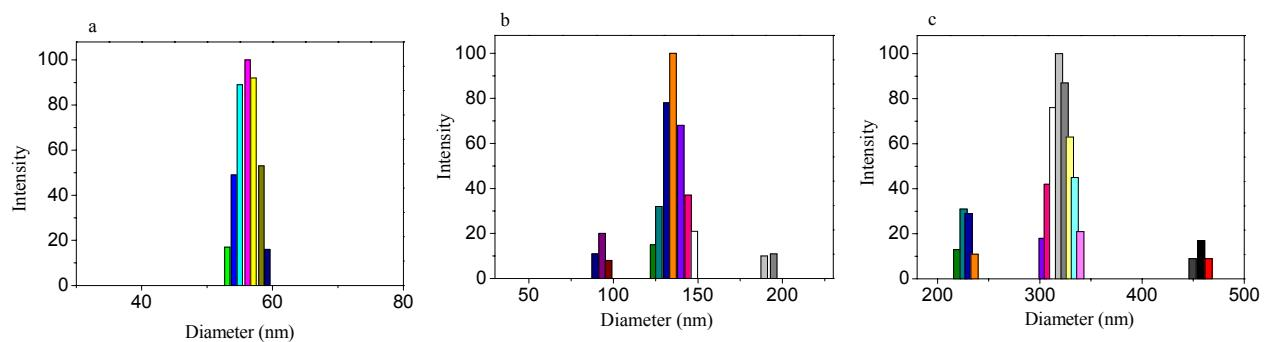
Fig. 6S. Particle size distributions of WCMs1000 with different morphologies, (a) monolayer WCMs1000, (b) compound WCMs1000 and (c) vesicle-like WCMs1000.
