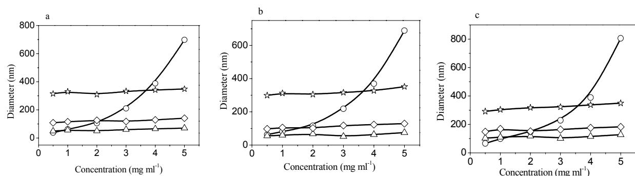
Fig. 5S. The particle size of O-B-EG micelles (○), monolayer WCMs (△), compound WCMs (◊) and vesicle-like WCMs(☆) with different molecular weight of PEG chains as an effect of micellar concentration, (a) PEG800, (b) PEG1000, (c) PEG 1500.
