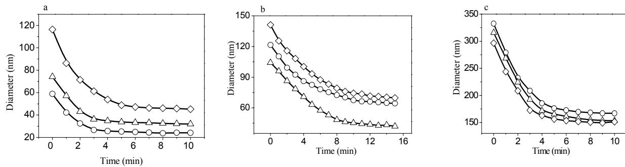
Fig. 7S. The shrinking speed of (a) monolayer WCMs, (b) compound WCMs and (c) vesicle-like WCMs with different molecular weight of PEG chains (○) PEG800, (△) PEG1000 (◊) PEG1500.
