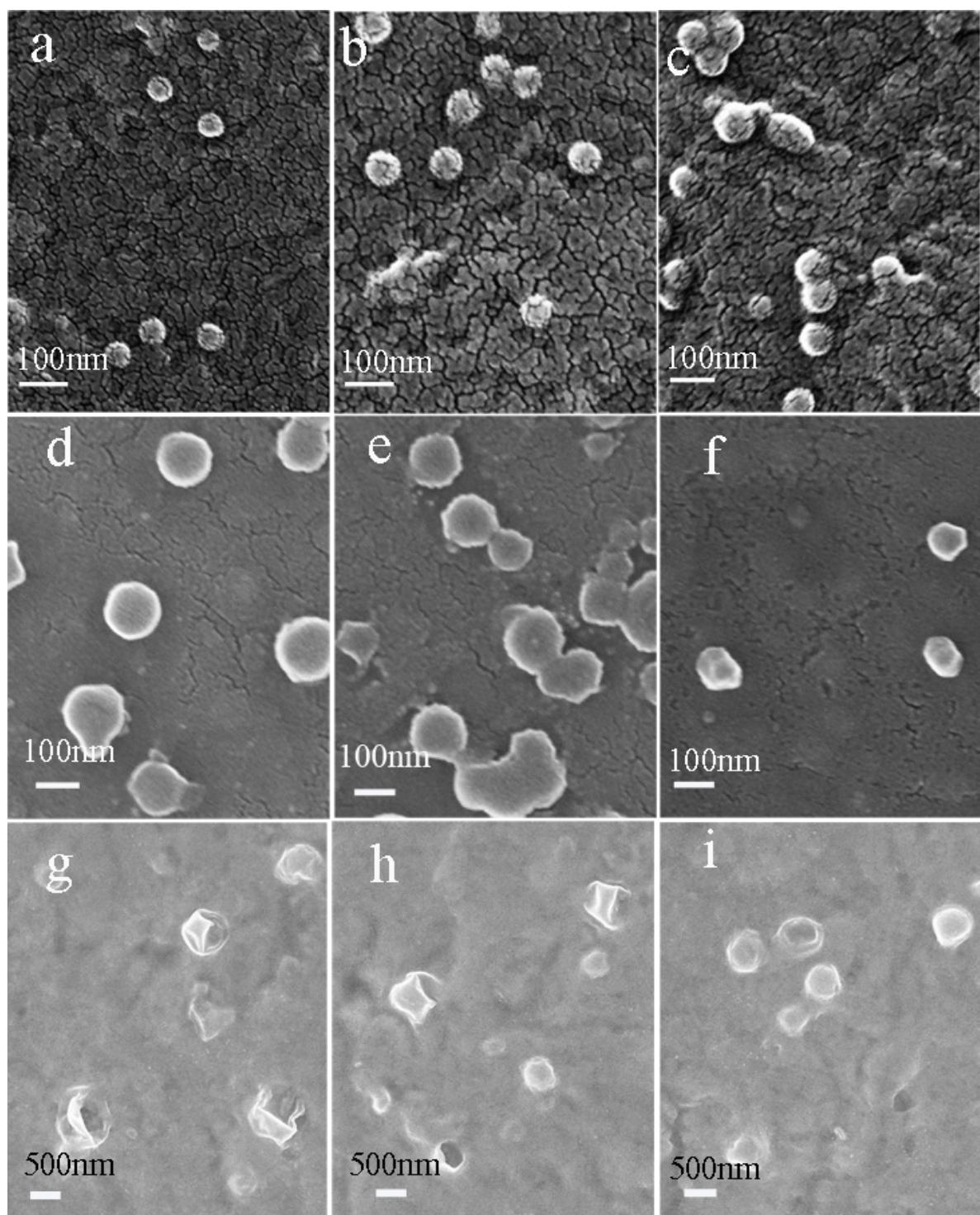
Fig. 3S. SEM images of (a) monolayer WCMs800, (b) monolayer WCMs1000, (c) monolayer WCMs1500, (d) compound WCMs800, (e) compound WCMs1000, (f) compound WCMs1500, (g) vesicle-like WCMs800, (h) vesicle-like WCMs1000 and (i) vesicle-like WCMs1500.
