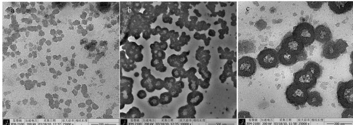
Fig. 4S. TEM images of O-B-EG1000 micelles obtained from 4.0 mg ml<sup>-1</sup> of O-B-EG1000 aqueous solution (a), WCMs1000 prepared from 3.0 mg ml<sup>-1</sup> of O-B-EG aqueous solution and WCMs1000 synthesized from 4.0 mg ml<sup>-1</sup> of O-B-EG aqueous solution (c).
