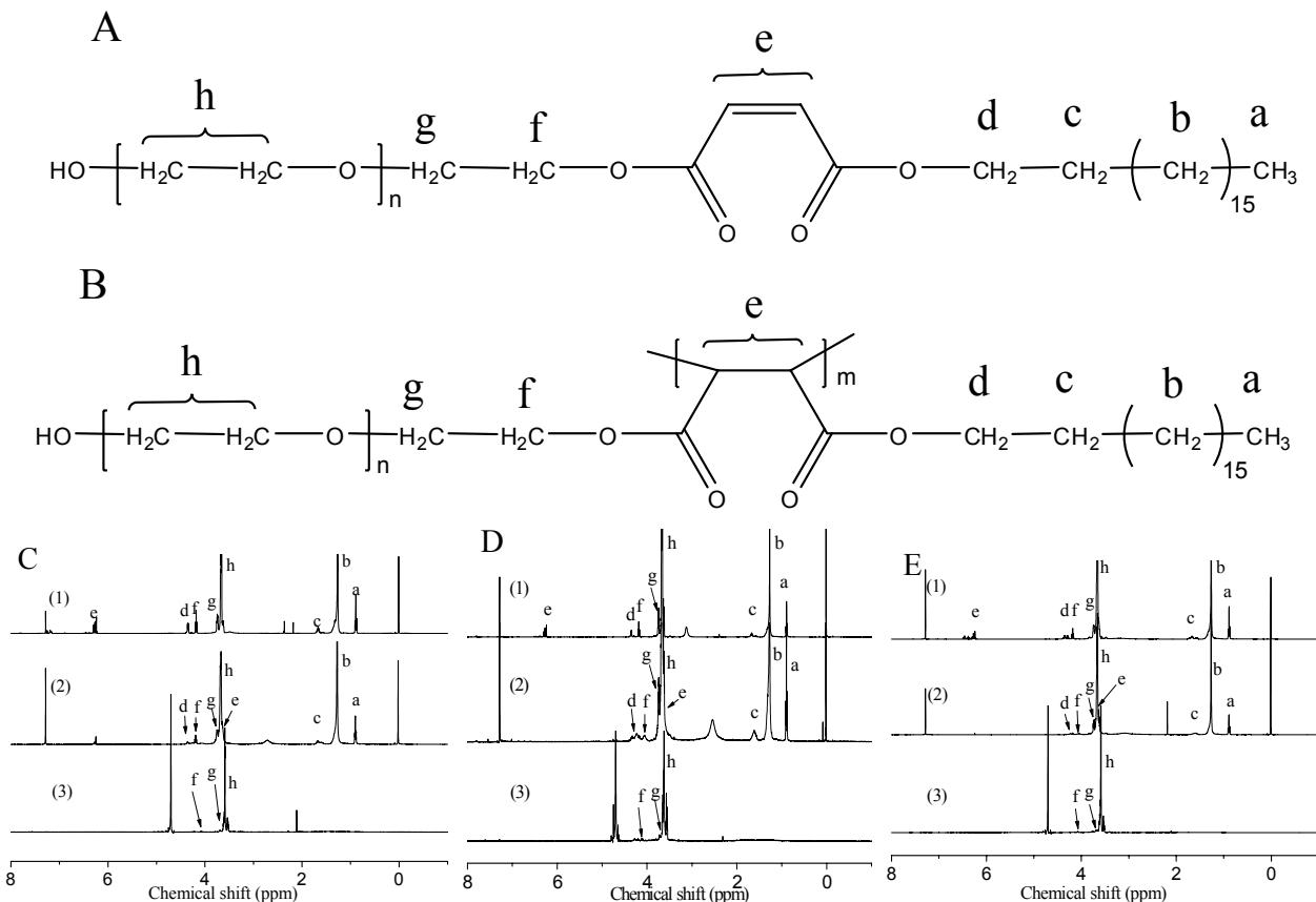
Fig. 1S. Chemical structure O-B-EG (A) and WCMs (B); <sup>1</sup>H NMR spectra of O-B-EG and WCMs with different molecular weight of PEG chains (C-1) O-B-EG800 in CDCl<sub>3</sub>, (C-2) WCMs800 in CDCl<sub>3</sub>, (C-3) WCMs800 in D<sub>2</sub>O, (D-1) O-B-EG1000 in CDCl<sub>3</sub>, (D-2) WCMs1000 in CDCl<sub>3</sub>, (D-3) WCMs1000 in D<sub>2</sub>O, (E-1) O-B-EG1500 in CDCl<sub>3</sub>, (E-2) WCMs1500 in CDCl<sub>3</sub>, and (E-3) WCMs1500 in D<sub>2</sub>O.
