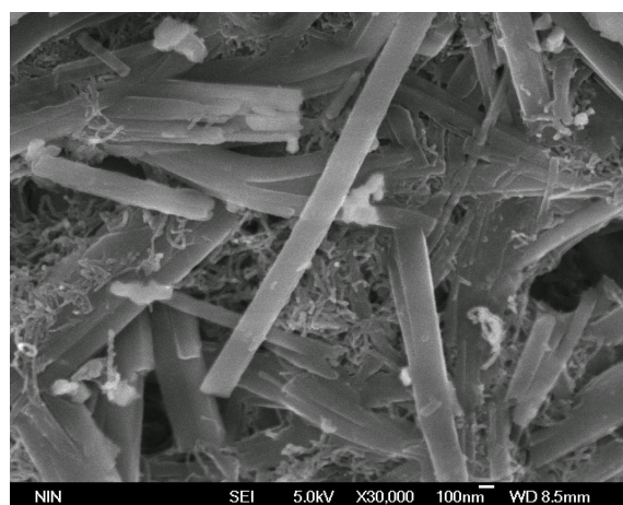
Fig. S3 SEM image of MWCNT-templated assemblies S1.
