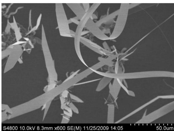
**Figure S3. SEM image of as-synthesized CdSe nanobelts on a silicon oxide substrate by chemical vapor deposition and used for making photo-sensors.**
