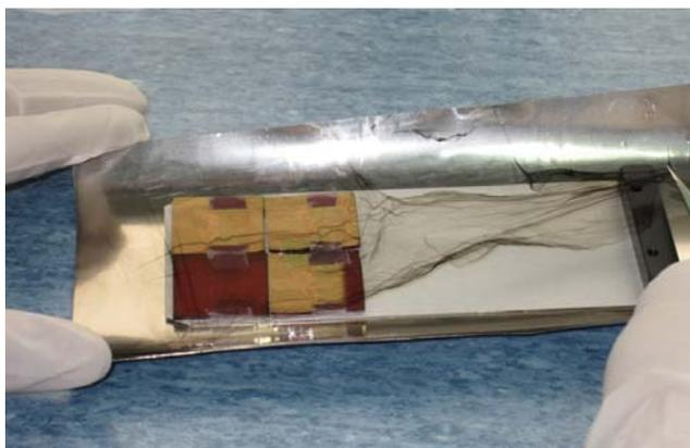
**Figure S1. Fabrication of CNT transparent electrode on the P3HT: PCBM layer.**
