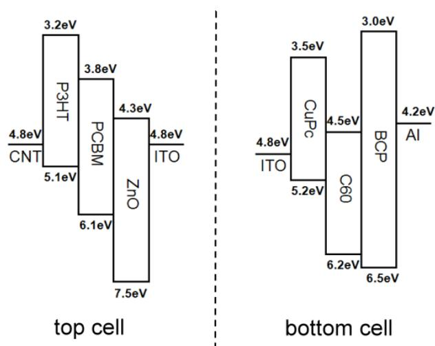
**Figure S2. Energy diagrams of the top and bottom cell in our tandem structure.**
