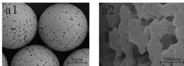
Fig.S4 SEM images of macro-porous beads from Baseline co. Ltd. (a1)  $\times 30000$ , (a2) the portion magnitude pictures of a single bead,  $\times 500000$
