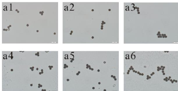
Fig.S2 cross-linked PSEMBs in solvent mixtures containing (a) 100 % isopropanol; (b) 5 % chloroform and 95 % isopropanol; (c) 20 % chloroform and 80 % isopropanol; (d) 40 % chloroform and 60 % isopropanol; (e) 60 % chloroform and 40 % isopropanol; (f) 100 % chloroform (vol/vol). The scale bar is 50  $\mu\text{m}$ .
