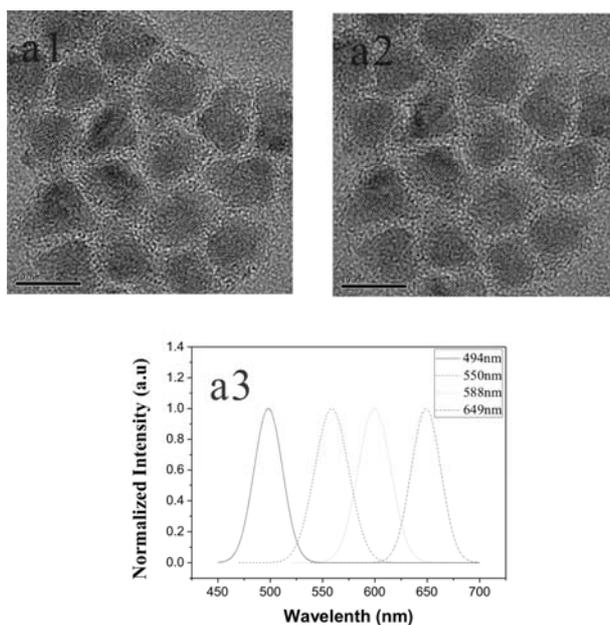
Fig.S3 TEM photographs of QDs (a1, a2) and PL spectra of  $\text{Cd}_x\text{Zn}_{1-x}\text{Se}_y\text{S}_{1-y}$  nanocrystals with emission wavelength of 494 nm, 550 nm, 588 nm and 649 nm (a3). The scale bar is 10 nm.
