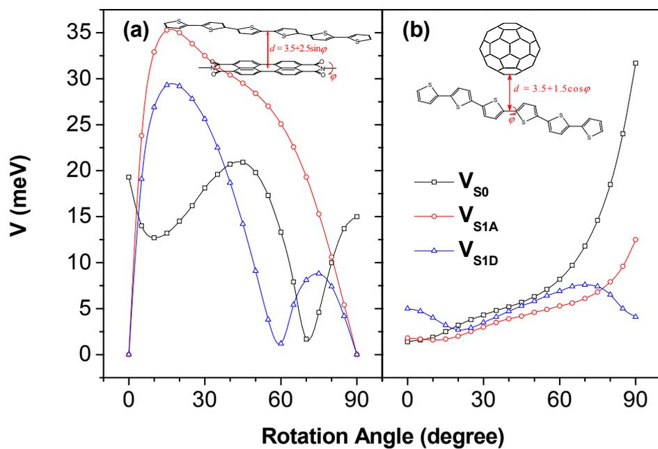
**Figure S3.** Electronic couplings to the lowest CT state for the ground state ( $V_{S0}$ ) and for the lowest local-excited singlet state on PDI or C<sub>60</sub> ( $V_{S1A}$ ) and on 6T ( $V_{S1D}$ ), as a function of the rotation angles along the long axis of PDI and the central carbon-carbon single bond of 6T, for complexes 6T/PDI and 6T/C<sub>60</sub>, respectively.
