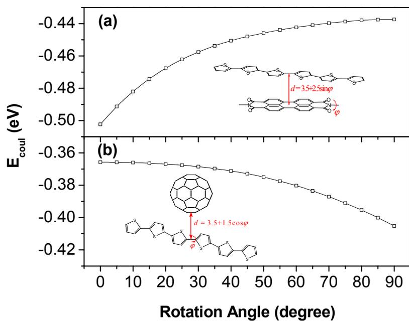
**Figure S2.** Calculated Coulomb energy of the lowest CT state as a function of the rotation angles along the long axis of PDI and the central carbon-carbon single bond of 6T for complexes 6T/PDI and 6T/C<sub>60</sub>, respectively.
