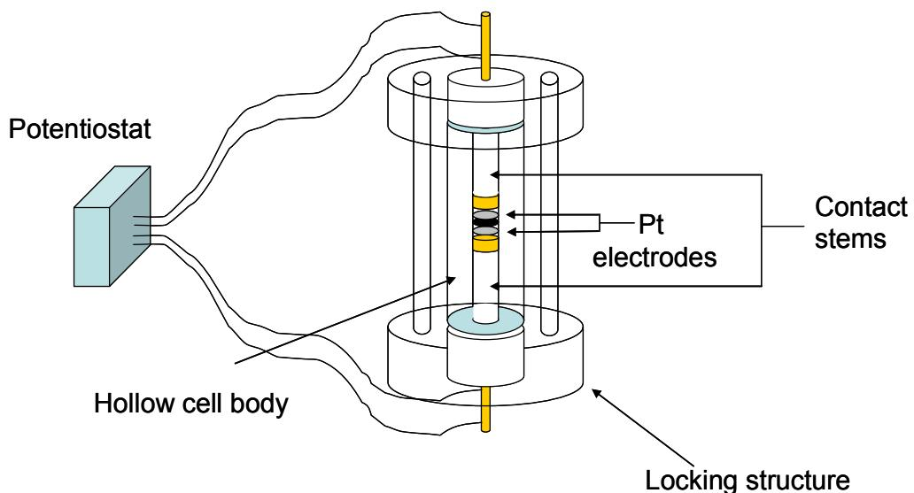
**Figure S2:** Schematic representation of the cell employed for resistivity measurements.
