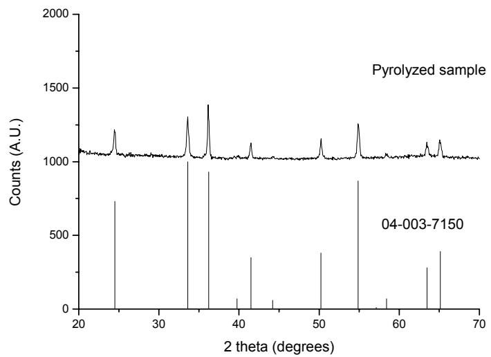
**Figure S3.** XRD Pattern of the pyrolyzed carbon composite fiber residue.
