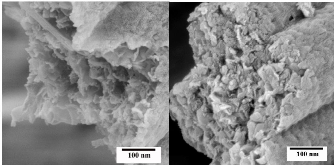
**Figure S8.** SEM images of the cross section of fibers treated at 1400°C after conductivity measurements.
