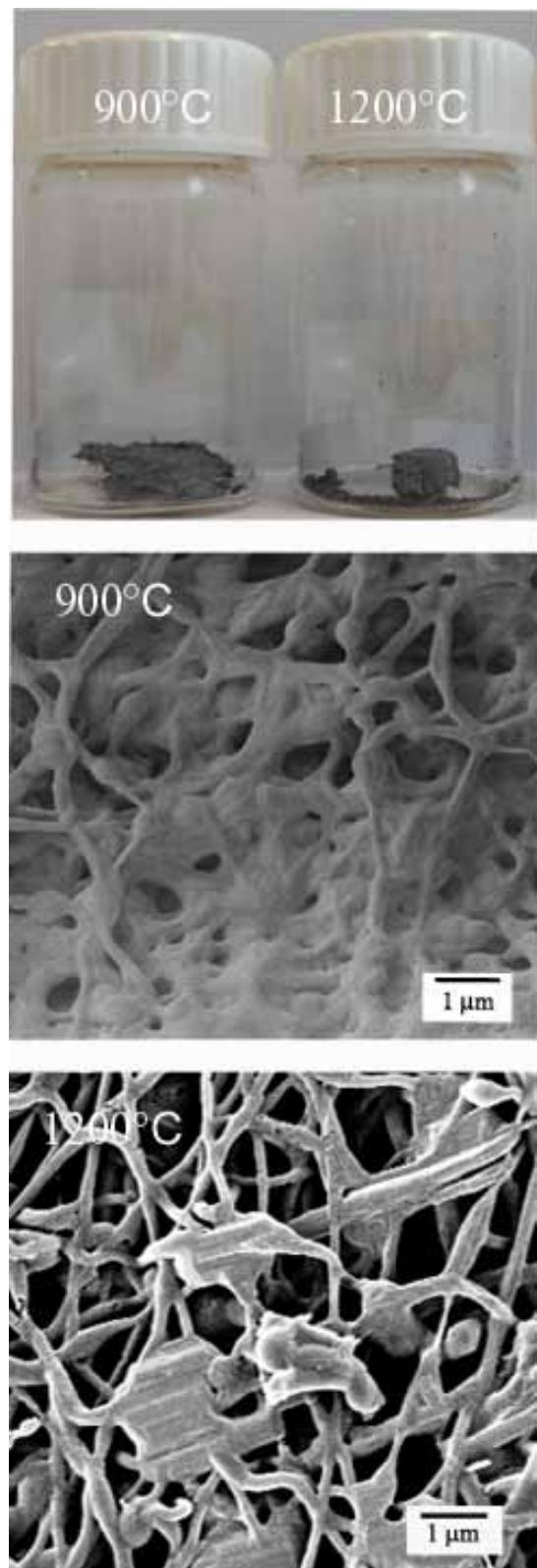
**Figure S4.** Images of samples calcined after brief exposition to high humidity conditions.
