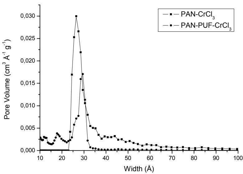
**Figure S7:** NLDFT Plots of the pore distributions from PAN-Cr and PAN-PUF-Cr at 1400°C.
