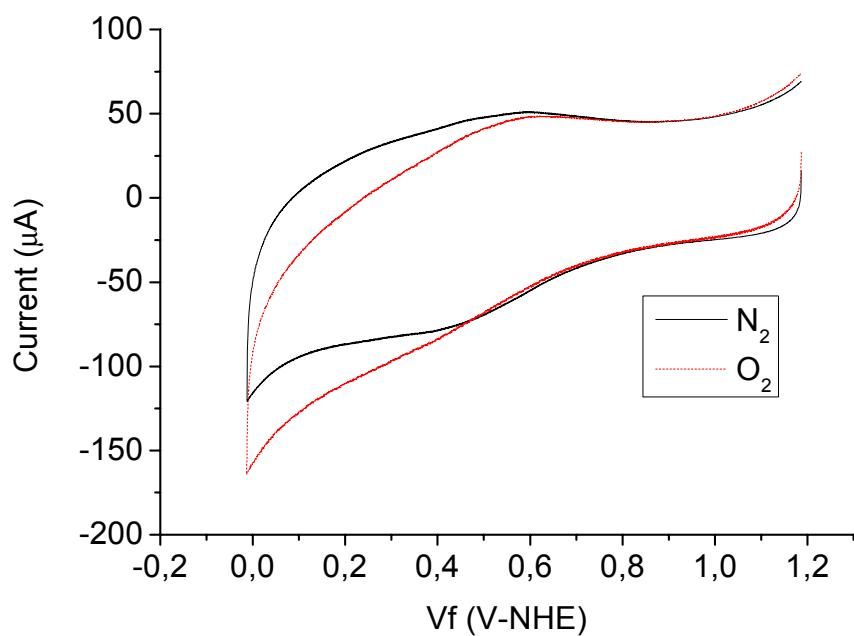
**Figure S9.** Cyclic voltammograms of the PUF containing composite in nitrogen saturated solution (black) and oxygen saturated solution (red).
