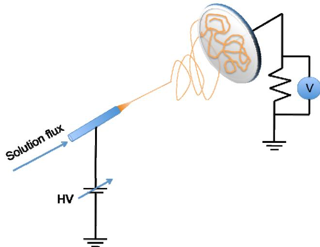
**Figure S1.** Schematization of the electrospinning device.
