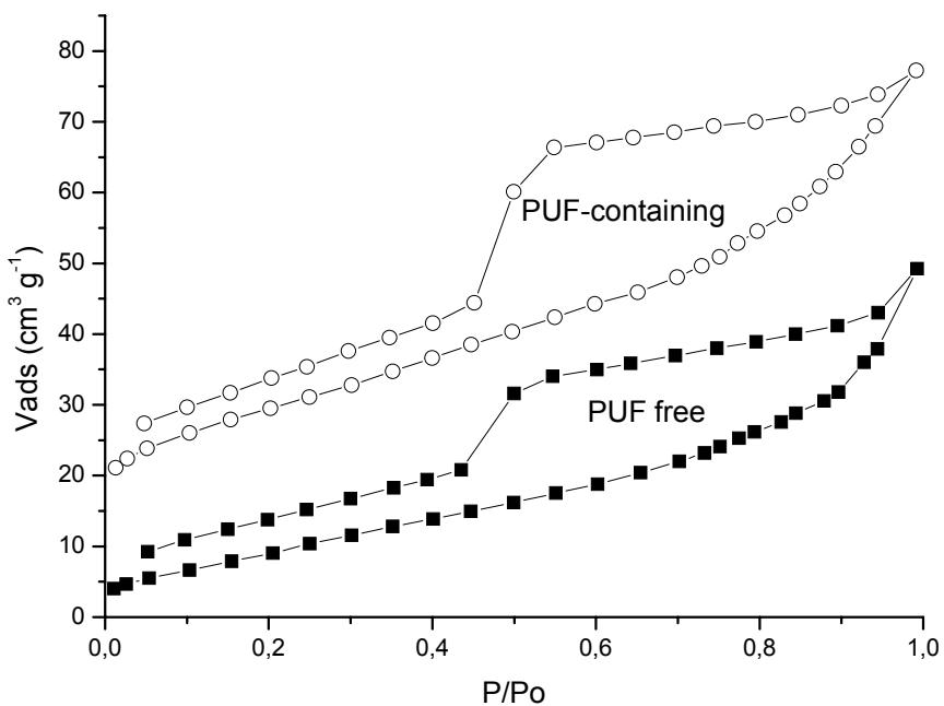
**Figure S6.** Nitrogen sorption isotherms of fibers calcined at 1400°C.
