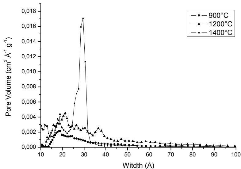
**Figure S5.** NLDFT plots of pore size distribution for PUF containing samples.
