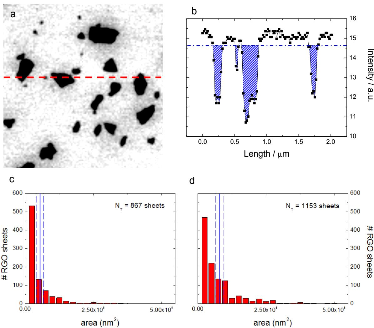
**Fig. S4** a) A SEM image and b) the profile corresponding to the red line traced in the 2D image by tracing a line. The threshold value is marked as a blue dash dotted line which identifies the sheets (blue regions) from the substrate. Frequency counts of the observed GO sheets for c)  $0.25 \text{ g}\cdot\text{L}^{-1}$  and d)  $= 0.5 \text{ g}\cdot\text{L}^{-1}$ . Mean values and corresponding error bars are represented with vertical blue lines.
