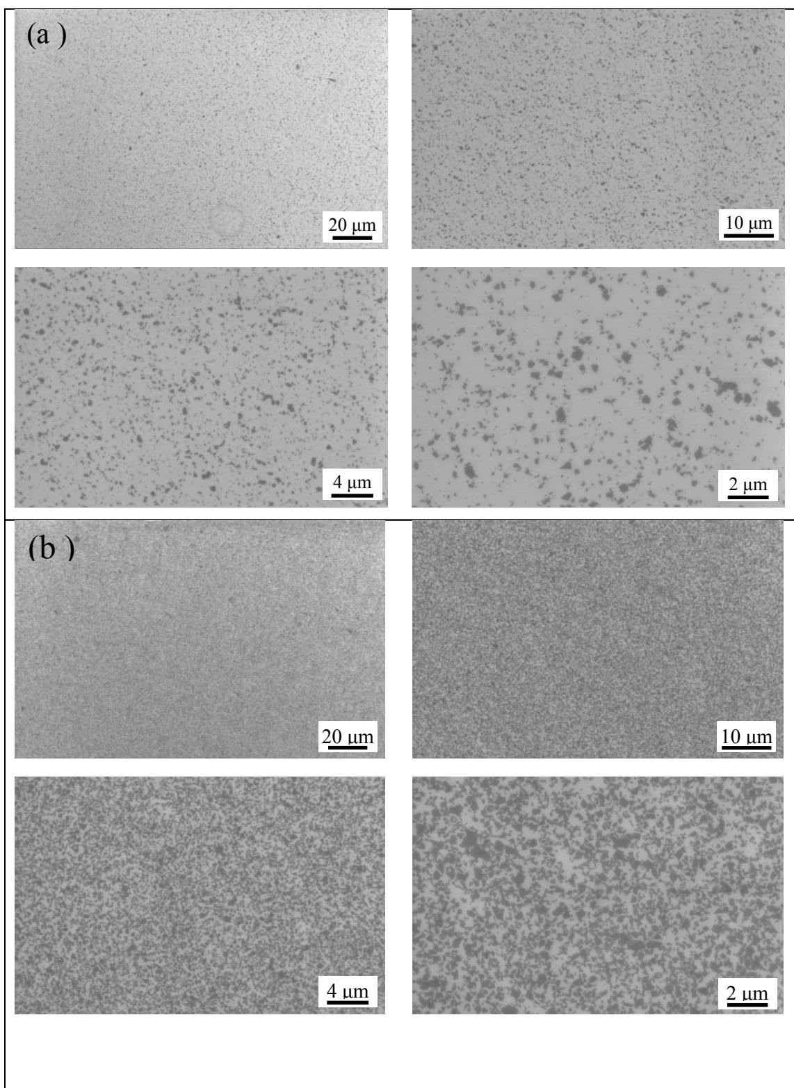
**Fig. S2** SEM images of graphene sheets obtained at different magnifications. (a)  $0.25 \text{ g}\cdot\text{L}^{-1}$  and (b)  $1 \text{ g}\cdot\text{L}^{-1}$  concentrations.
