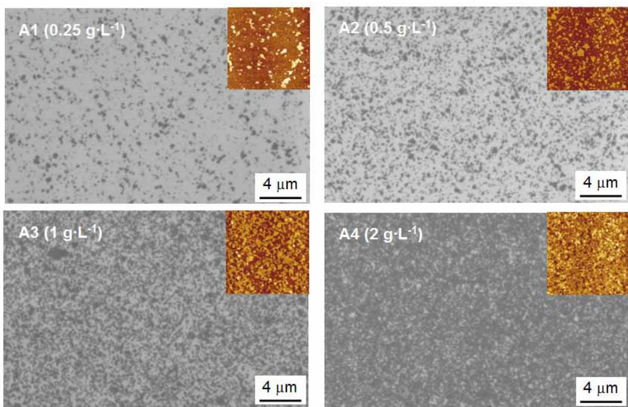
**Fig. S1** SEM images of graphene sheets obtained at different concentrations: (A1) =  $0.25 \text{ g L}^{-1}$ , (A2) =  $0.5 \text{ g L}^{-1}$ , (A3) =  $1 \text{ g L}^{-1}$ , and (A4) =  $2 \text{ g L}^{-1}$ . In the insets, an AFM image of each sample reported with the same data scale. Z range of inserts = 3 nm.
