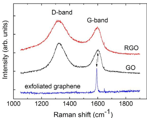
Fig. S3. The Raman spectra of GO, RGO and exfoliated graphene in the region of D- and G-band. The spectra were normalized to the G-band intensity. The arrows visualize the shift of the G-band.
