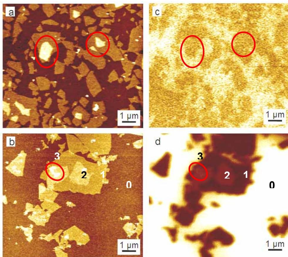
**Fig. S5** AFM images of (a) GO and (b) RGO sheets on native SiO<sub>x</sub> and corresponding (c,d) KPFM images. Z ranges: (a) = 4 nm, (b) = 6 nm, (c) = 150 mV and (d) 250 mV.
