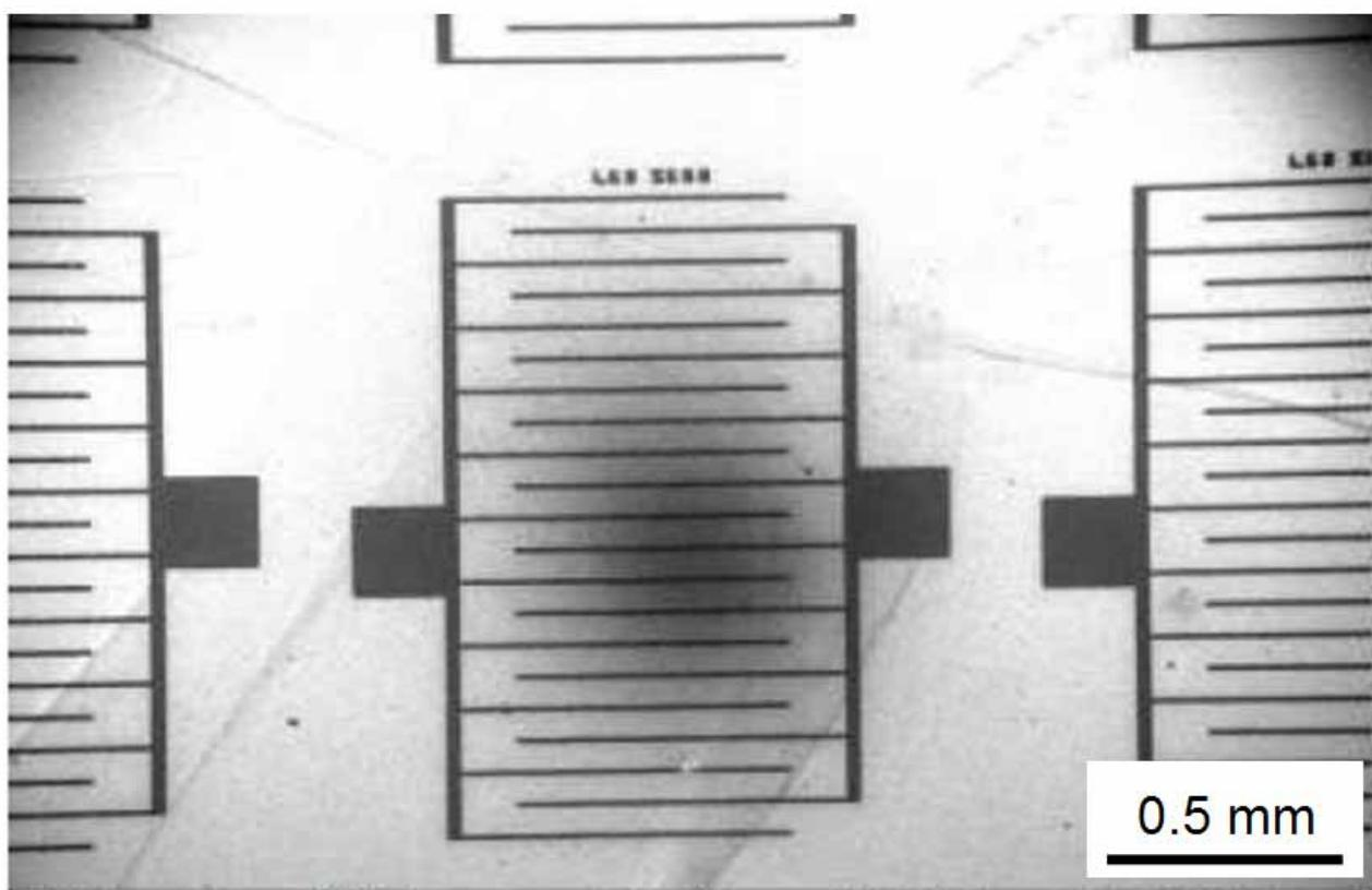
**Fig. S6** SEM image of the transistor architecture used for FET measurements (W/L = 200, channel length of 60  $\mu\text{m}$ )
