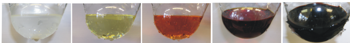
Figure S2. Photographs of the OFC-1A synthesis in solution (0.2 g 14DAB in 60 ml Ethanol/Toluene (5:1)), taken directly after the addition of different amounts of \text{SiCl}_4 (from the left to the right image: 0 ml, 8 ml, 10 ml, 12 ml, 12 ml after 30 min).
