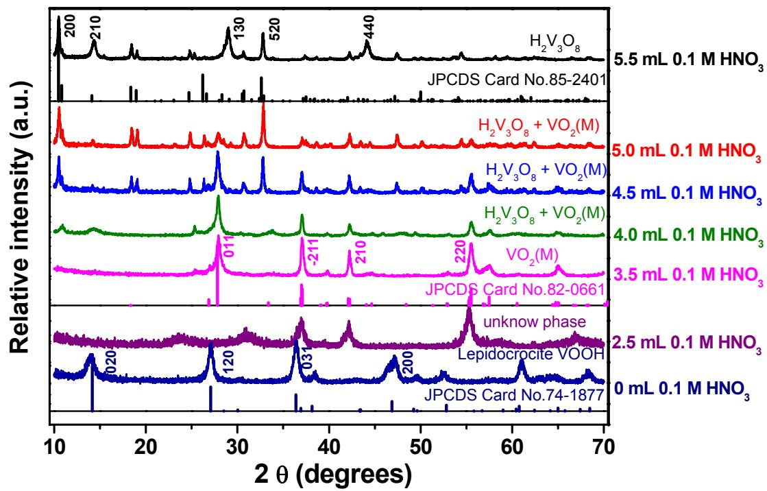
**Figure S5.** XRD patterns of the as-obtained samples when different amount of  $\text{HNO}_3$  was involved keeping other reaction parameters constant.
