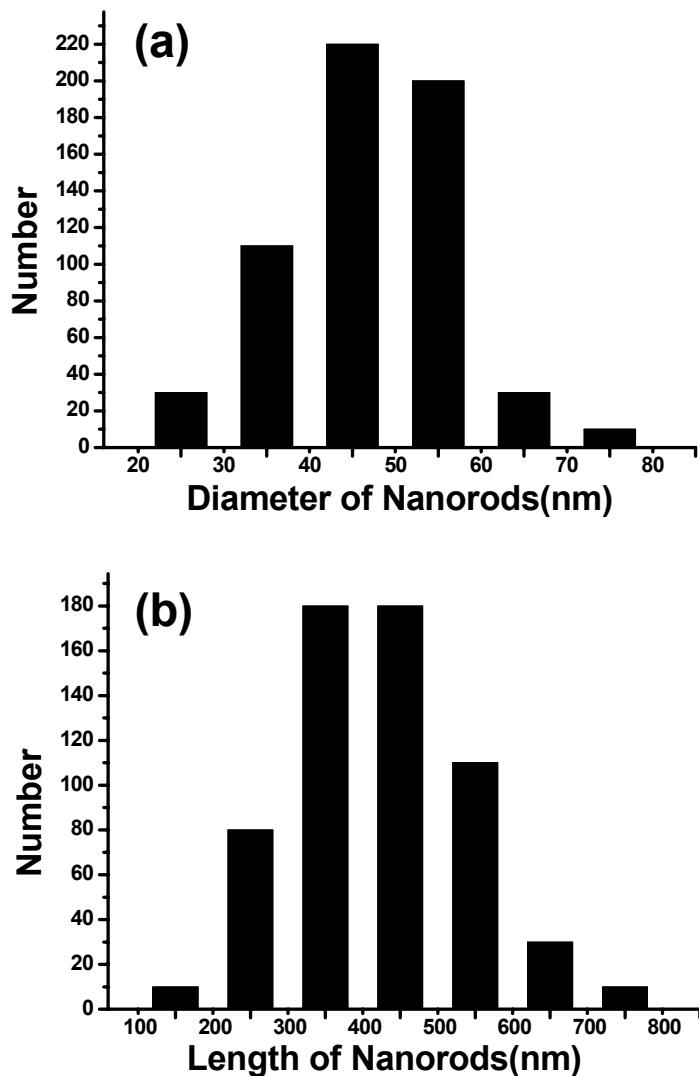
**Figure S3.** The diameter and length size distribution histogram of the as-obtained nanorods for monoclinic  $\text{VO}_2(\text{M})$ , showing that the nanorod outlook with the diameter size ranging from 30 nm to 120 nm and lengths up to 400 - 800 nm in large scale.
