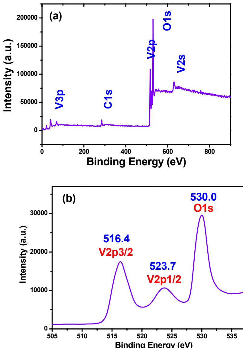
**Figure S2.** (a) The survey XPS spectrum of synthetic monoclinic VO<sub>2</sub>(M) product, where only the V and O can be found while the carbon peak at 284.6 eV was taken as reference. (b) the high resolution XPS (HRXPS) for V2p and O1s region.
