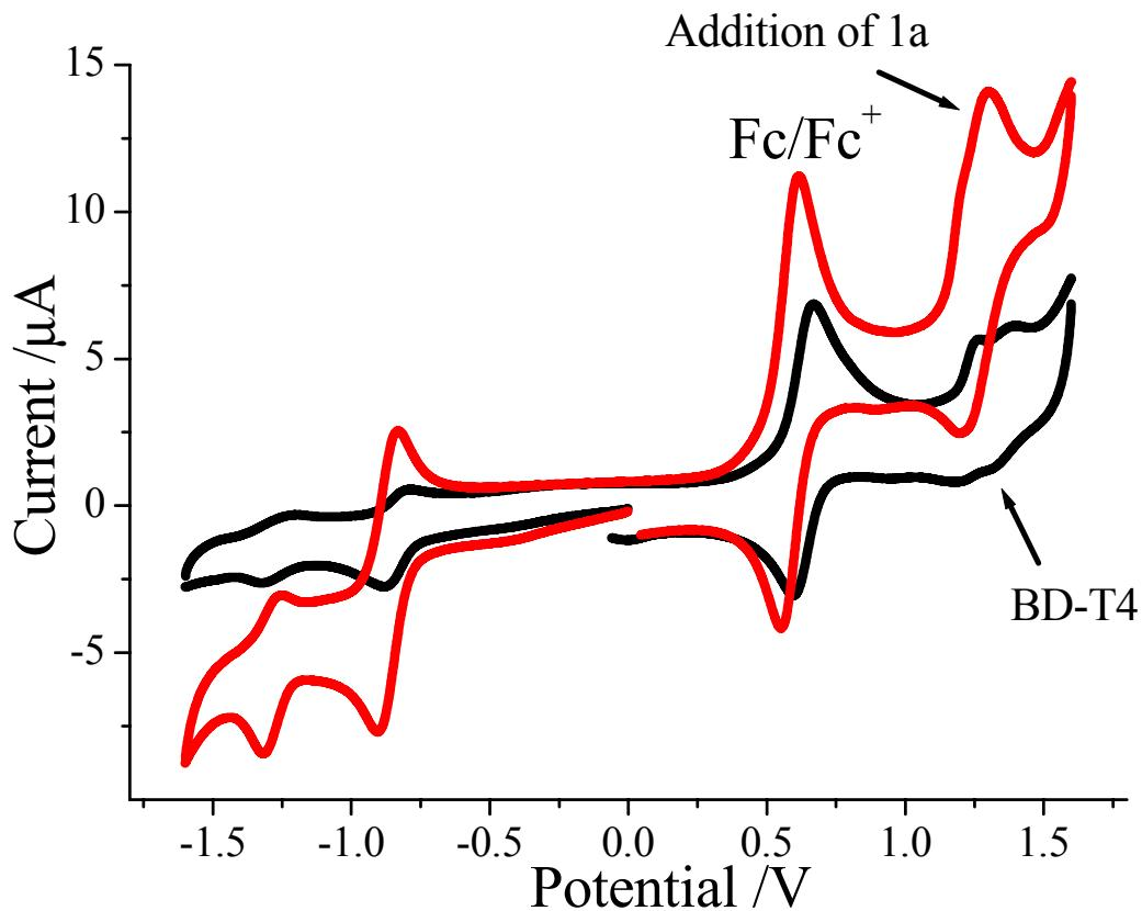
S6. Cyclic voltammograms for **BD-T4** (dark) and in the presence of **1a** (red) in dry N<sub>2</sub>-purged CH<sub>3</sub>CN (0.2 M TBATFB) at a Pt working electrode and Ag wire reference. Scan rate = 100 mVs<sup>-1</sup>.
