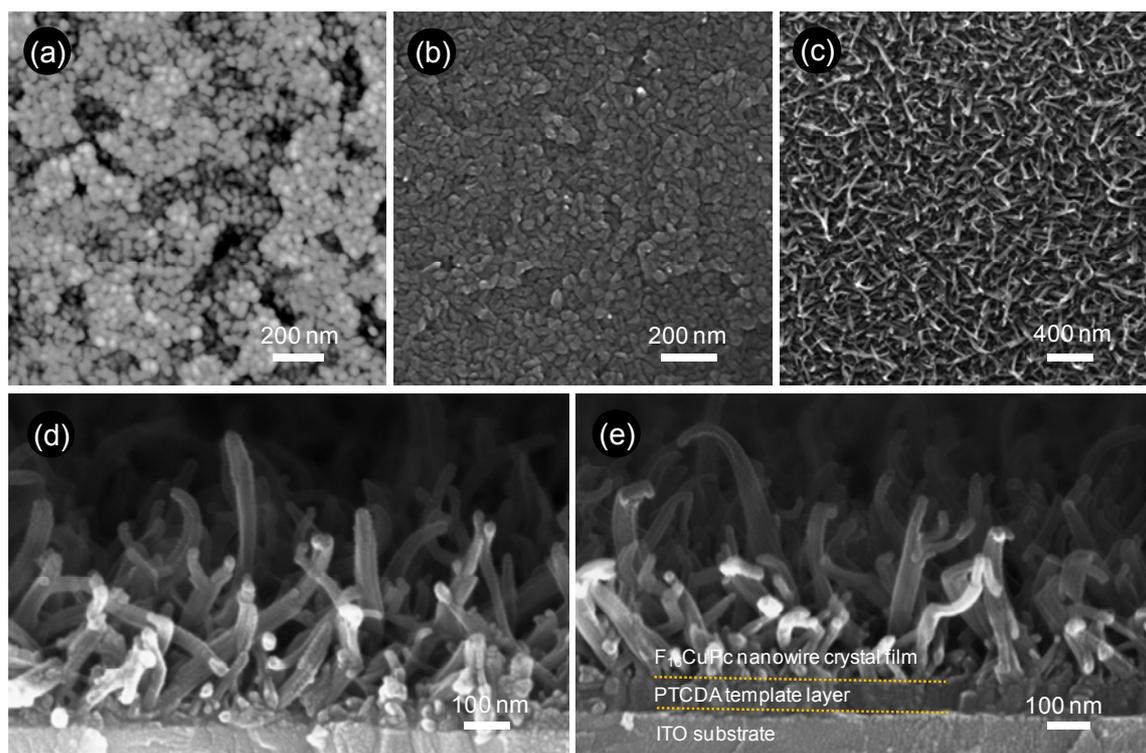
**Figure 1** Morphology of the PTCDA template layer and the  $F_{16}CuPc$  pristine and templated films grown on ITO: (a) PTCDA (5 nm), (b)  $F_{16}CuPc$  (35 nm), (c)  $F_{16}CuPc$  (75 nm)/PTCDA (5 nm), (d) cross-sectional image of  $F_{16}CuPc$  (75 nm)/PTCDA (5 nm), (e) cross-sectional image of  $F_{16}CuPc$  (75 nm)/PTCDA (70 nm).
