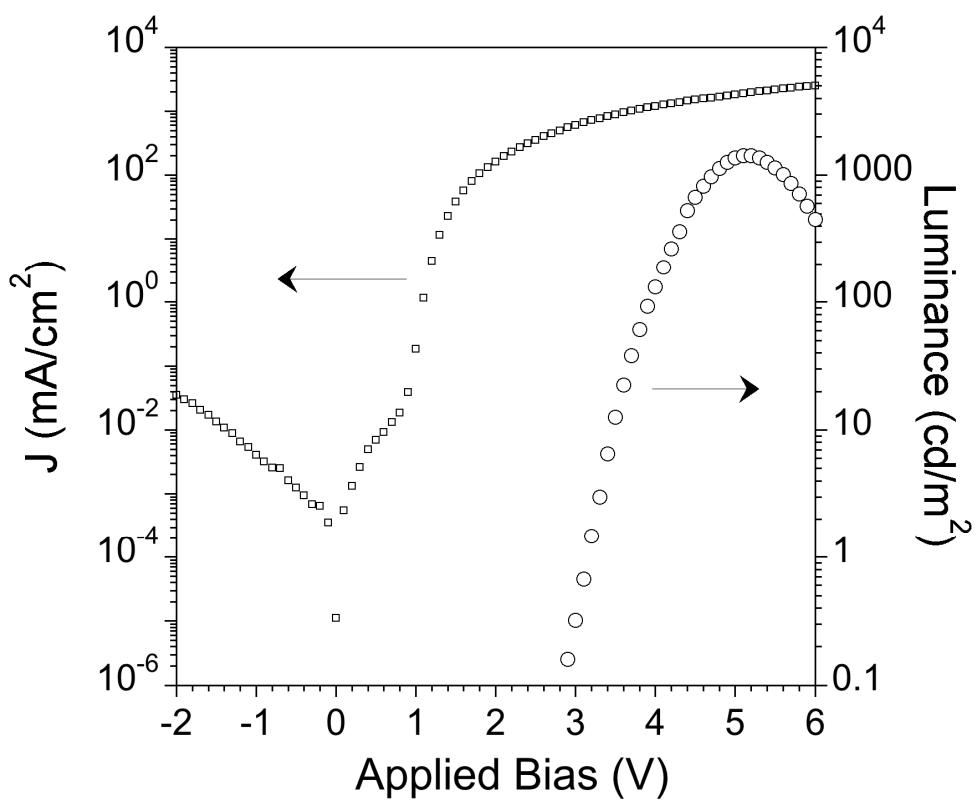
**Figure S1.** Device performance of ITO/F8BT/MoO<sub>3</sub>/Au.
