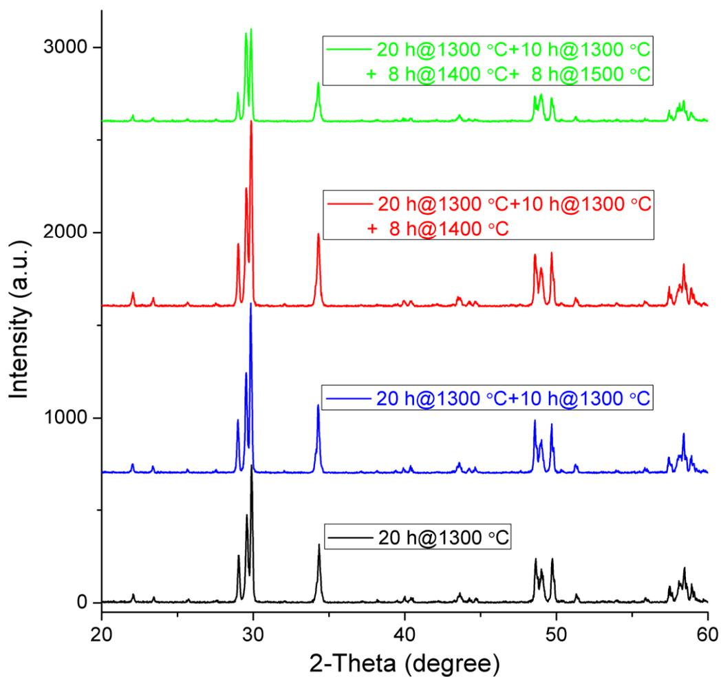
XRD patterns of  $Y_6MoO_{12}:Eu$  synthesized at different calcination temperatures and holding times.
