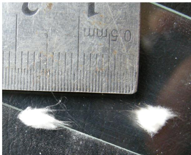
Figure S3. Photograph of the  $\beta$ -Si<sub>5</sub>AlON<sub>7</sub> nanobelts thermal treated at 1450°C for 2 hours
