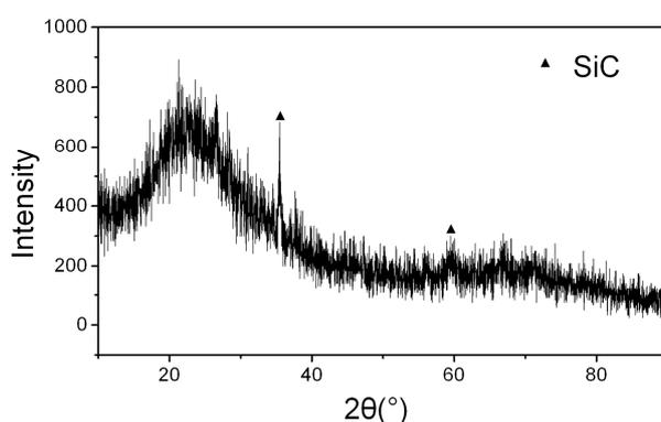
Figure S4 XRD pattern recorded from SiONCH-Al annulus debris thermal treated at 1000° C for 2 hours
