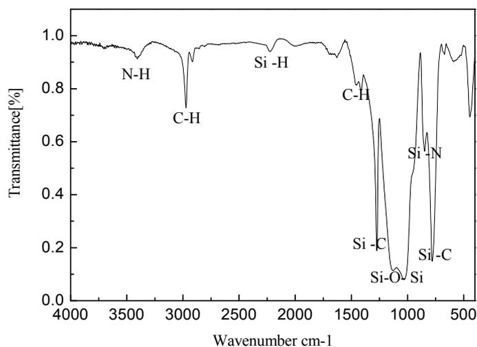
Figure S1. FT- IR spectrum of SiONCH sol-gel
