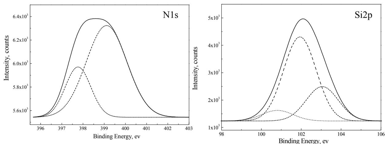
Figure S2. XPS spectra of N1s and Si2p of SiONCH sol-gel
