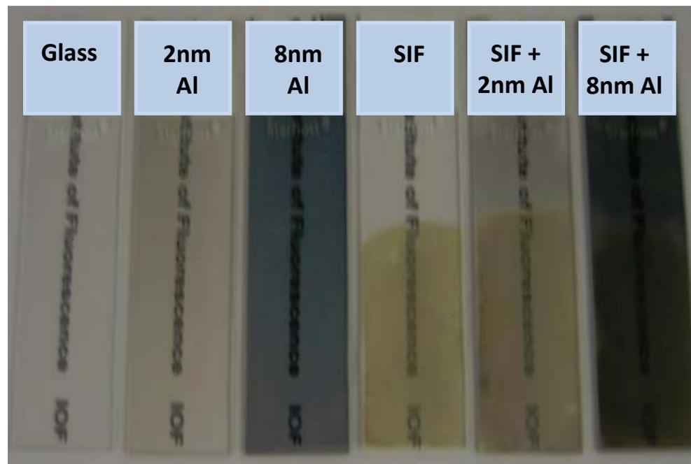
**Figure 1S.** Photographs of metal depositions on glass slides
