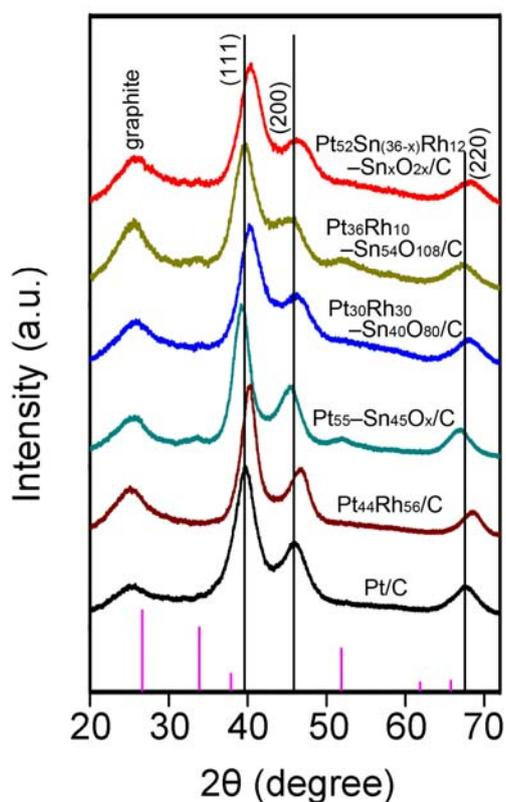
**Figure S2.** XRD patterns of as-made  $\text{Pt}_{52}\text{Sn}_{(36-x)}\text{Rh}_{12}\text{-Sn}_x\text{O}_{2x}/\text{C}$ ,  $\text{Pt}_{36}\text{Rh}_{10}\text{-Sn}_{54}\text{O}_{108}/\text{C}$  and  $\text{Pt}_{30}\text{Rh}_{30}\text{-Sn}_{40}\text{O}_{80}/\text{C}$ ,  $\text{Pt}_{55}\text{-Sn}_{45}\text{O}_x/\text{C}$ ,  $\text{Pt}_{44}\text{Rh}_{56}/\text{C}$ , and Pt/C (ETEK) carbon supported
