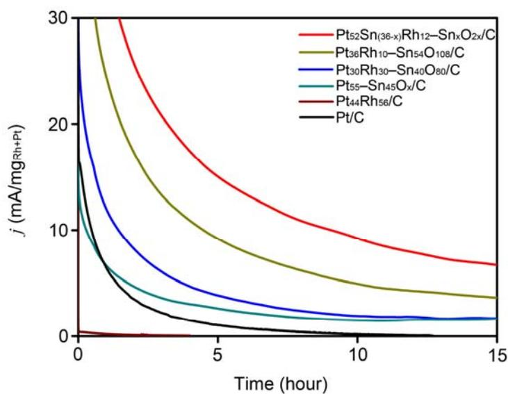
**Figure S6.** IT curves of Pt<sub>52</sub>Sn<sub>(36-x)</sub>Rh<sub>12</sub>-Sn<sub>x</sub>O<sub>2x</sub> /C, Pt<sub>36</sub>Rh<sub>10</sub>-Sn<sub>54</sub>O<sub>108</sub>/C, Pt<sub>30</sub>Rh<sub>30</sub>-Sn<sub>40</sub>O<sub>80</sub>/C, Pt<sub>55</sub>-Sn<sub>45</sub>O<sub>x</sub> /C, Pt<sub>44</sub>Rh<sub>56</sub>/C, and Pt/C (Etek) in ethanol-containing acid solution.
