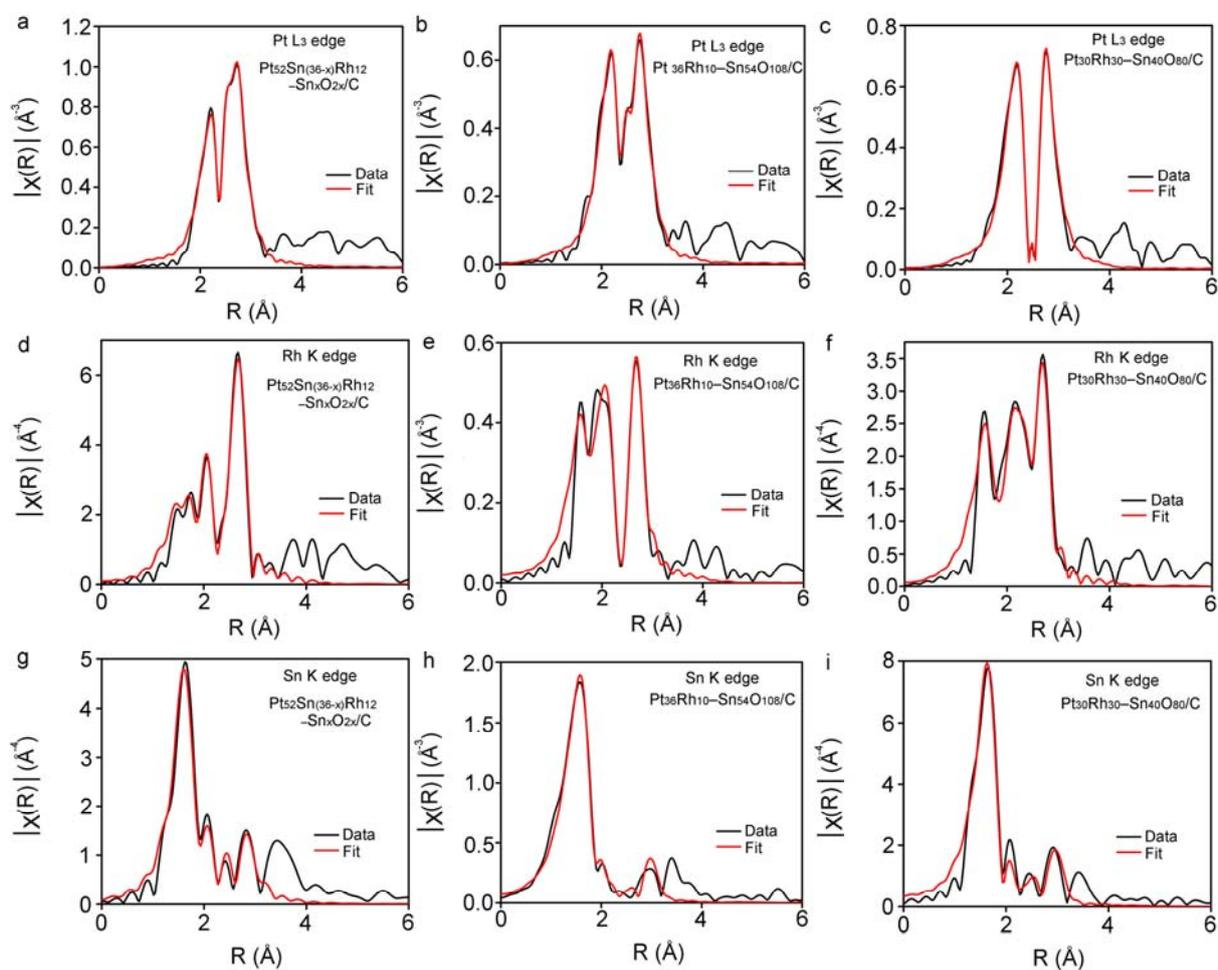
**Figure S4.** Fourier transform magnitudes of EXAFS data of the (a, b, c) Pt L<sub>3</sub> edge, (d, e, f) Rh K edge, (g, h, i) Sn K edge, for three carbon-supported Pt/Sn/Rh ternary catalysts.
