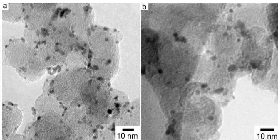
**Figure S7.** TEM images of carbon-supported (a)  $\text{Pt}_{30}\text{Rh}_{30}\text{-Sn}_{40}\text{O}_{80}$  and (b)  $\text{Pt}_{36}\text{Rh}_{10}\text{-Sn}_{54}\text{O}_{108}$  catalysts.
