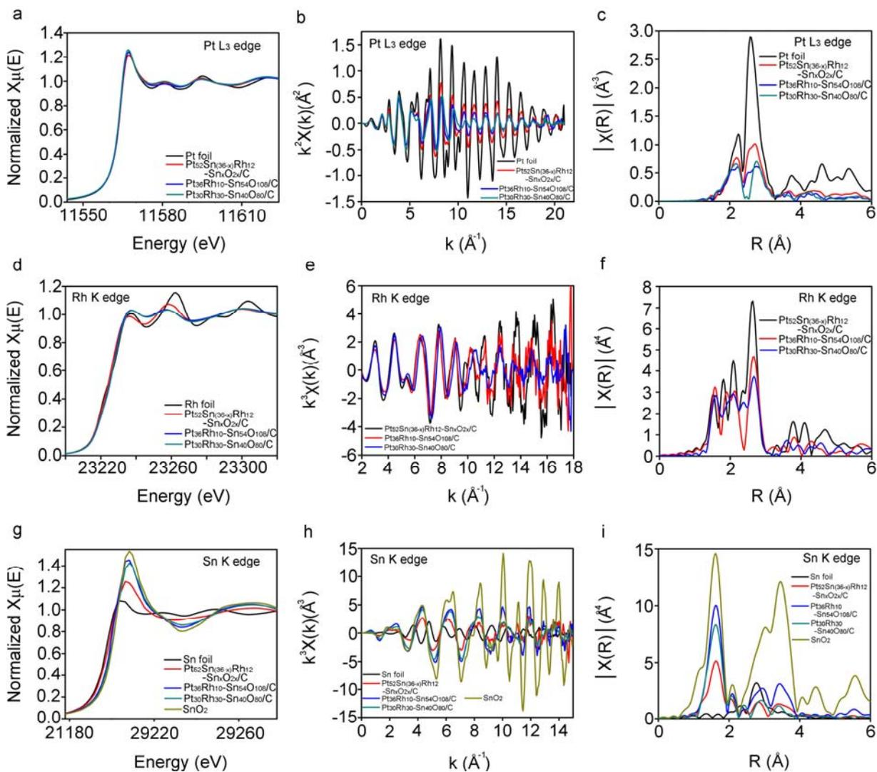
**Figure S3.** XANES and EXAFS spectra for three Pt/Sn/Rh catalysts: Pt<sub>52</sub>Sn<sub>(36-x)</sub>Rh<sub>12</sub>-Sn<sub>x</sub>O<sub>2x</sub>/C, Pt<sub>36</sub>Rh<sub>10</sub>-Sn<sub>54</sub>O<sub>x</sub>/C and Pt<sub>30</sub>Rh<sub>30</sub>-Sn<sub>40</sub>O<sub>x</sub>/C : (a, b, c) Pt L3 edge; (d, e, f) Rh K edge; (g, h, i) Sn K edge. For k-space and R-space data, k<sup>2</sup>-weighting is used for Pt L3 data and k<sup>3</sup>-weighting for Rh K edge and Sn K edge.
