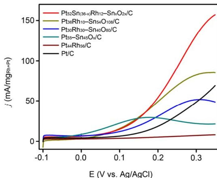
**Figure S5.** CV curves of Pt<sub>52</sub>Sn<sub>(36-x)</sub>Rh<sub>12</sub>-Sn<sub>x</sub>O<sub>2x</sub> /C, Pt<sub>36</sub>Rh<sub>10</sub>-Sn<sub>54</sub>O<sub>108</sub>/C, Pt<sub>30</sub>Rh<sub>30</sub>-Sn<sub>40</sub>O<sub>80</sub>/C, Pt<sub>55</sub>-Sn<sub>45</sub>O<sub>x</sub> /C, Pt<sub>44</sub>Rh<sub>56</sub>/C, and Pt/C (Etek) in ethanol-containing acid solution.
