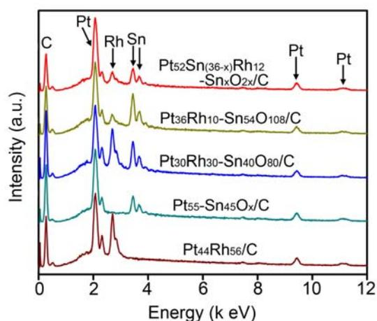
**Figure S1.** EDS spectra of as-made  $\text{Pt}_{52}\text{Sn}_{(36-x)}\text{Rh}_{12}\text{-Sn}_x\text{O}_{2x}/\text{C}$ ,  $\text{Pt}_{36}\text{Rh}_{10}\text{-Sn}_{54}\text{O}_{108}/\text{C}$  and  $\text{Pt}_{30}\text{Rh}_{30}\text{-Sn}_{40}\text{O}_{80}/\text{C}$ ,  $\text{Pt}_{55}\text{-Sn}_{45}\text{O}_x/\text{C}$ , and  $\text{Pt}_{44}\text{Rh}_{56}/\text{C}$  carbon supported nanoparticles.
