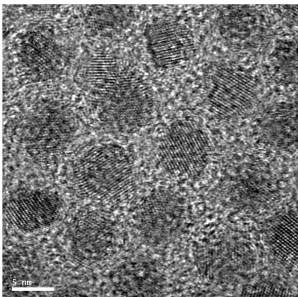
**Figure S3.** HR-TEM image of PbSe/CdSe HNCs after heating in diphenylether at 200 °C. Core/shell structures are difficult to identify, but nevertheless bi-hemisphere HNCs are also not present.
