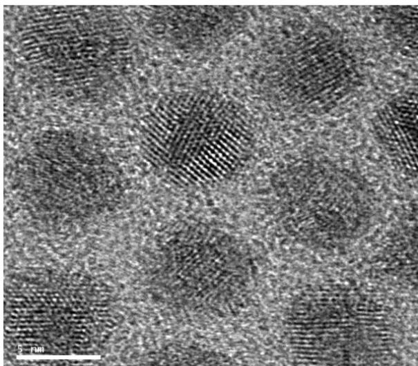
**Figure S2.** HR-TEM image of PbSe/CdSe HNCs after heating in diphenylether at 150 °C. The HNCs still possess a core/shell structure.
