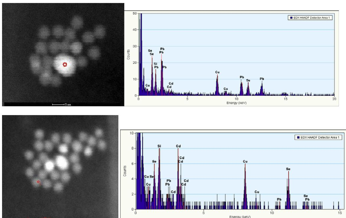
**Figure S4.** STEM images (right) and EDX analysis (left) of PbSe/CdSe HNCs heated in diphenylether at 220 °C. The red spots indicate the area on which the EDX analyses were done.
