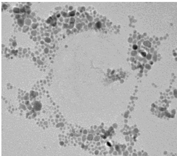
**Figure S5.** TEM image of PbSe/CdSe HNCs after heating in diphenylether at 240 °C.
