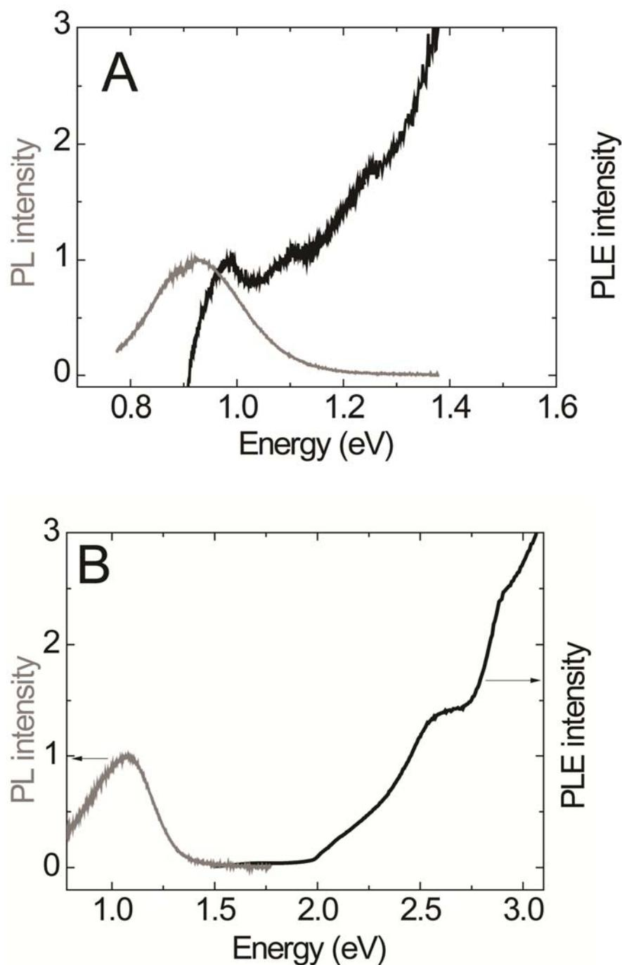
**Figure S6.** Photoluminescence (PL, grey line) and PL Excitation (PLE, black line) spectra of: (A) PbSe/CdSe core/shell QDs with a total diameter of 5.6 nm and 3.6 nm diameter core; and (B) PbSe/CdSe "peacock eye"-like bi-hemisphere HNCs obtained by thermal annealing of the sample shown in (A) at 160 °C under vacuum ( $10^{-6}$  mbar) in a rotary evaporator (see Figure 8 in the main text for illustrative HR-TEM images).
