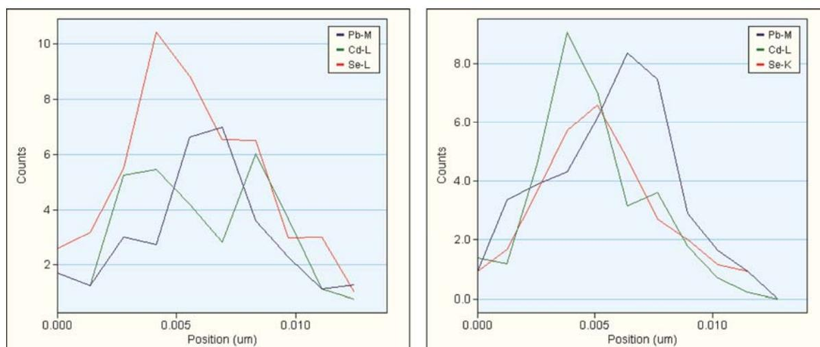
**Figure S1.** EDX analysis of two different PbSe/CdSe HNCs heated for 1.5 h at 160°C under vacuum ( $10^{-6}$  mbar) in a Schlenk line.
