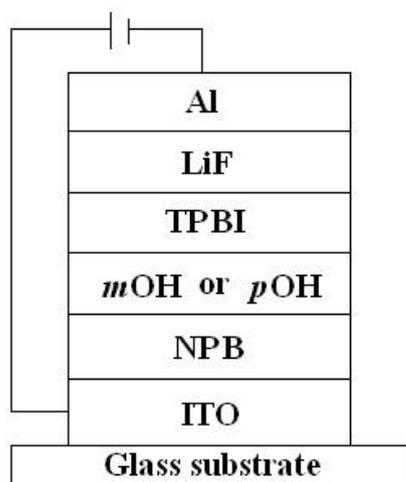
**Fig. S4.** Structure of devices for these derivatives
