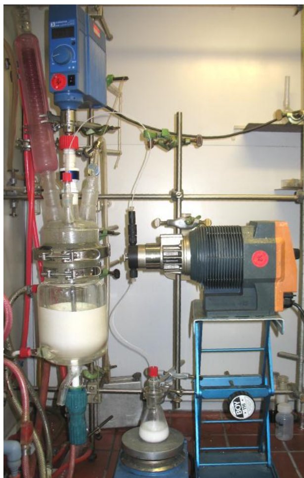
Figure S2: 1 litre stirred tank reactor
