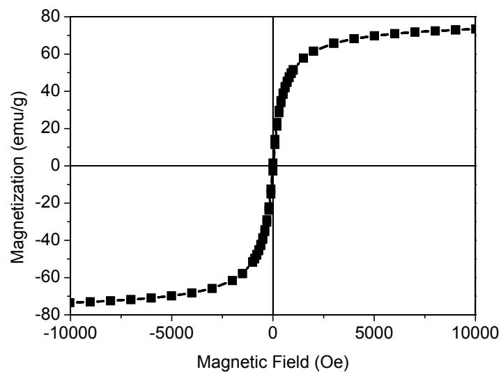
**Fig. S1** Field-dependent magnetization curves of  $\text{Fe}_3\text{O}_4$  nanoparticles at 300 K.
