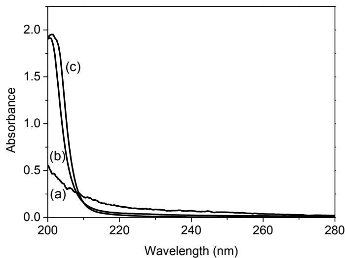
**Fig. S4** UV-vis spectra of (a) PDDA (0.01 mol/L), (b) BTAC (0.20 mol/L), (c) NaCl (0.25 mol/L).
