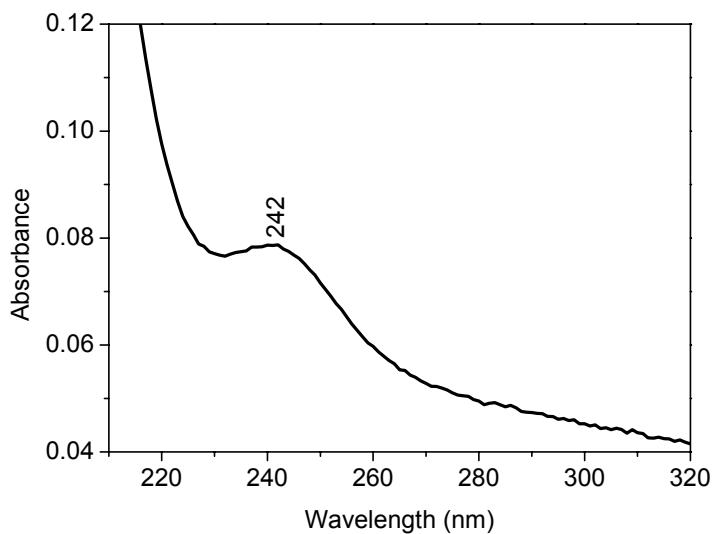
**Fig. S5** UV-vis spectrum of a TTAC-functionalized quartz plate after Hg(II) adsorption with a counterpart before Hg(II) adsorption as a reference.
