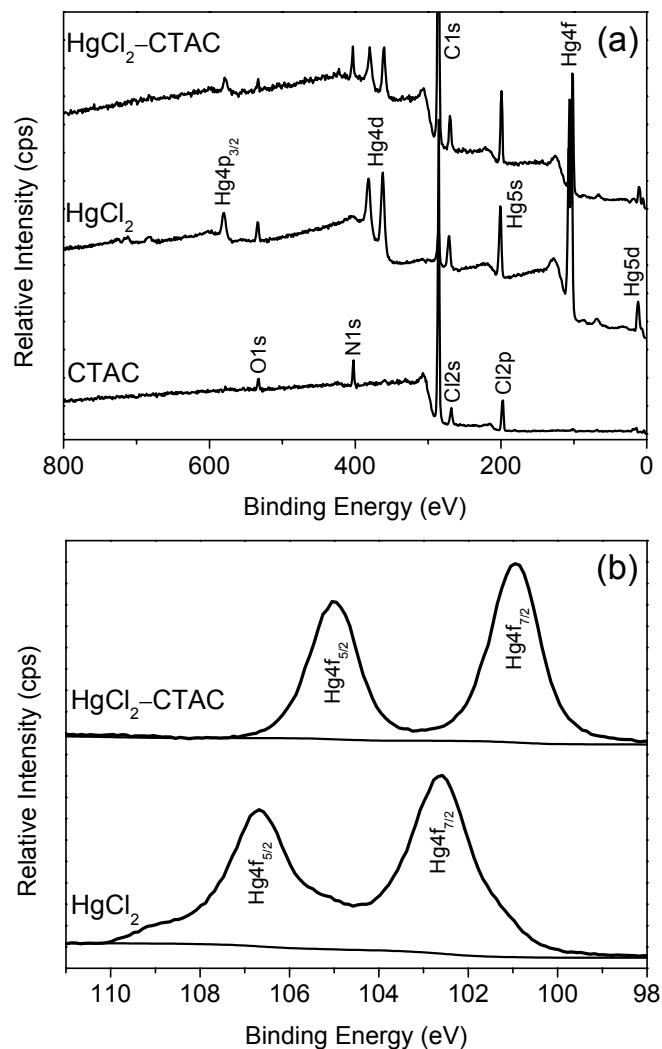
**Fig. S6** XPS spectra of CTAC,  $\text{HgCl}_2$ , and CTAC complex with  $\text{HgCl}_2$ : (a) survey scans; (b) high-resolution scans in the regions of  $\text{Si}2p$  and  $\text{Hg}4f$  binding energies
