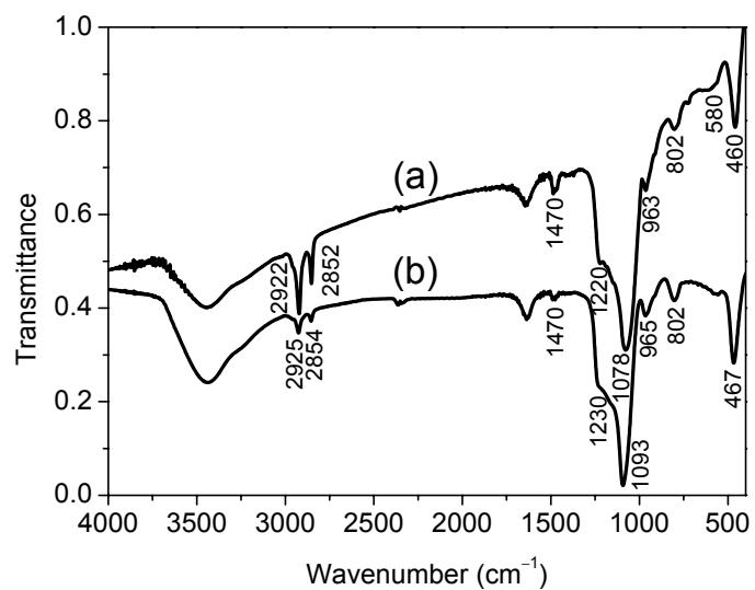
**Fig. S3** FTIR spectra of AMMS: (a) before surfactant extraction; (b) after surfactant extraction.
