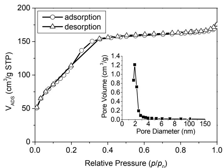
**Fig. S2** Nitrogen adsorption–desorption isotherms of AMMS. The inset shows pore size distribution of AMMS.
