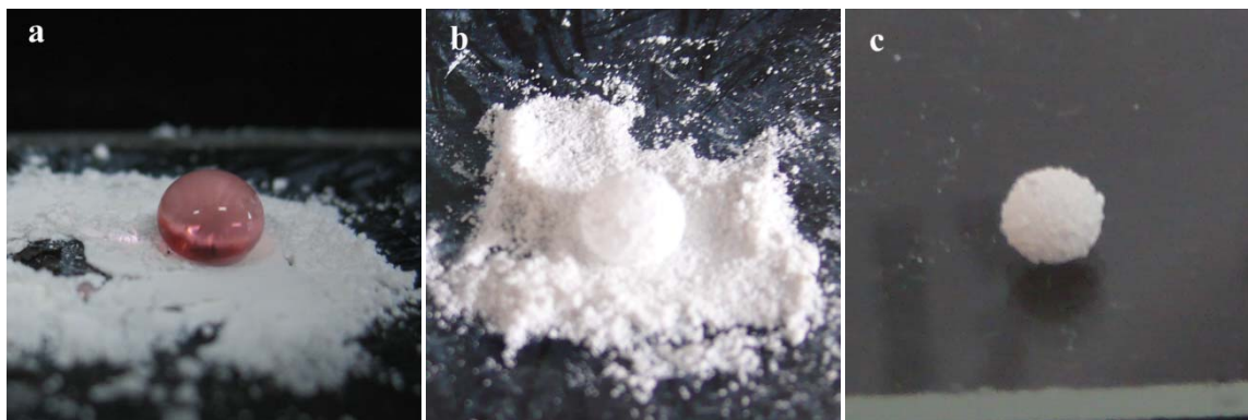
Figure S2. 50 \mu L colored water droplet rest on the sticky superhydrophobic materials (a), water droplet was coated with a lay of the sticky materials through rolling over the Ph-20-TM materials powder (b) and the coated water droplet rest on the hydrophilic glass flake (c).
