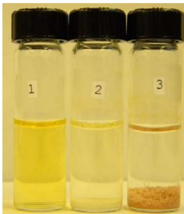
**Figure S13.** Pictures of Fe(III) chloride solution with ES-HU (3) and ES-NCO (2) samples in comparison to that of Fe(III) chloride solution only(1).
