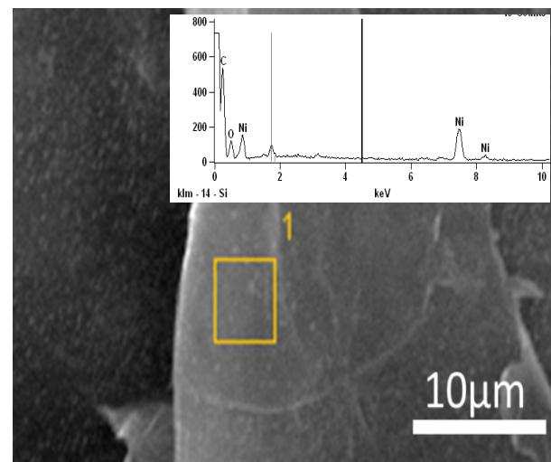
**Figure S2.** EDS spectrum of the as-prepared GNS/NiO sandwich membrane
