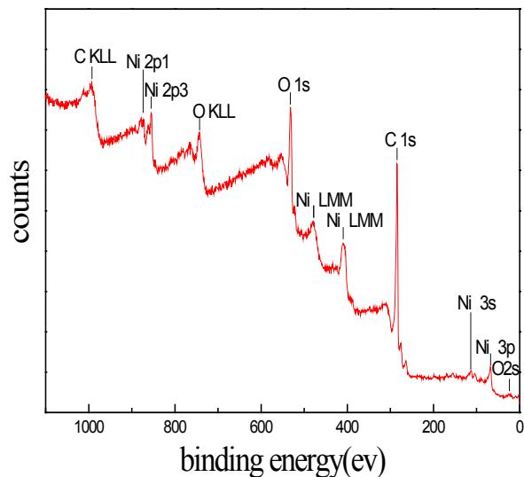
**Figure S1.** XPS wide-scan spectrum of the as-prepared GNS/NiO sandwich membrane
