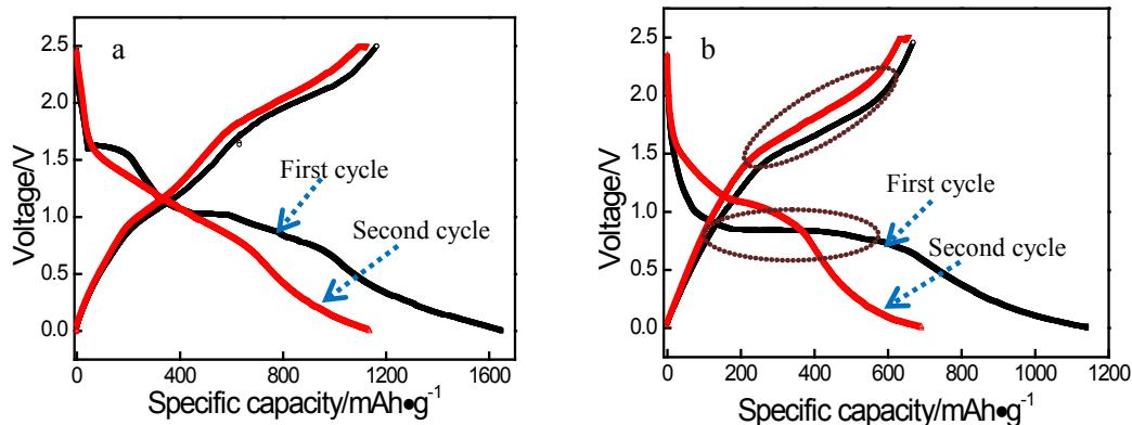
**Figure S6.** Charge-discharge (current density: 20 mA/g) profiles of sandwich membranes ((a), GNS/Co<sub>3</sub>O<sub>4</sub>; (b), GNS/Fe<sub>3</sub>O<sub>4</sub>) that were used as the anodes of Li-ion battery packs. For a larger current density (100 mA/g, not shown here), the discharge capacities of the above membranes are 550 and 480 mAh/g for the first cycle and still remain 490 and 420 mAh/g respectively after 40 cycles.
