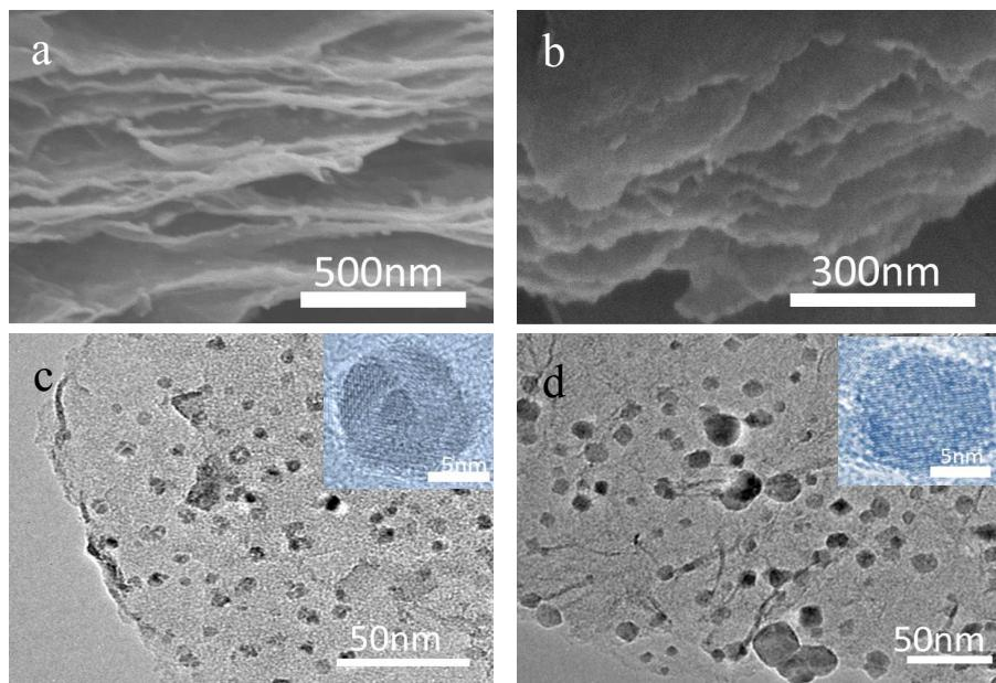
**Figure S5.** SEM images of GNS/Co<sub>3</sub>O<sub>4</sub> (a) and GNS/Fe<sub>3</sub>O<sub>4</sub> (b) sandwich membranes; TEM images of GNS/Co<sub>3</sub>O<sub>4</sub> (c) and GNS/Fe<sub>3</sub>O<sub>4</sub> (d) sandwich membranes. The overlays of (c) and (d) respectively represent the high-resolution TEM images of Co<sub>3</sub>O<sub>4</sub> and Fe<sub>3</sub>O<sub>4</sub> NPs.
