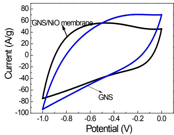
**Figure S4.** CV profiles of GNS/NiO membrane and GNS at the scan rate of 500 mV/s.
