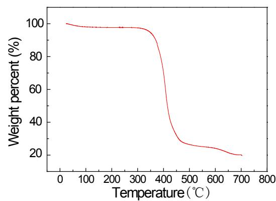
**Figure S3.** TG profile of the as-prepared GNS/NiO sandwich membrane
