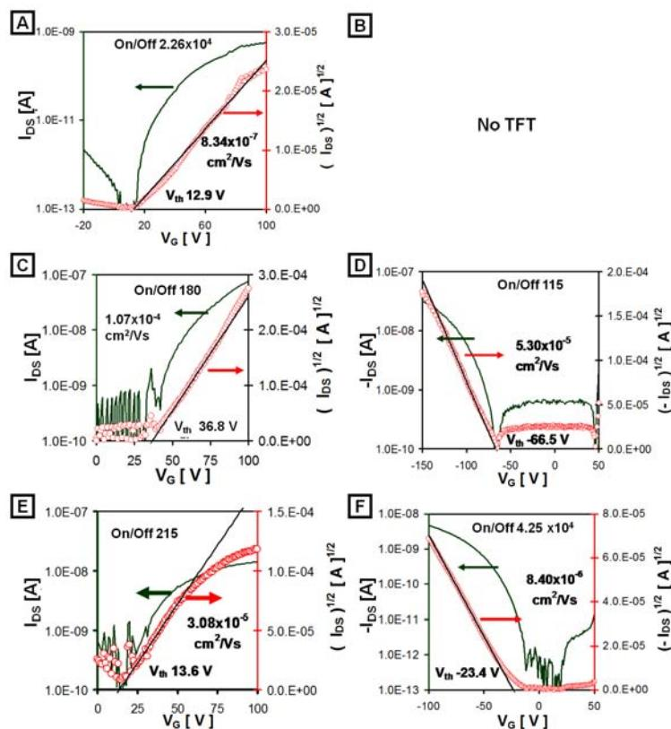
**Figure S2.** Performance of top-contact thin-film transistors fabricated from **1c** (A-B), **1a** (C-D) and **1b** (E-F). Plots A, C and E were measured inside a nitrogen environment, while the rest were measured in ambient conditions. Mobility is higher and threshold voltage is closer to zero for devices tested in nitrogen. W/L is 20 and L = 50  $\mu\text{m}$  in all cases. The drain-source voltage,  $V_{ds}$  is + 100.0 V for panels A,C and E, is -150.0 V for panel D and -100.0 for panel F.
