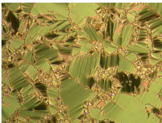
Fig 4. Micrographic texture of LCG-triester 8-PNP-O12 in a 15 \mu m thick liquid crystal cell.
