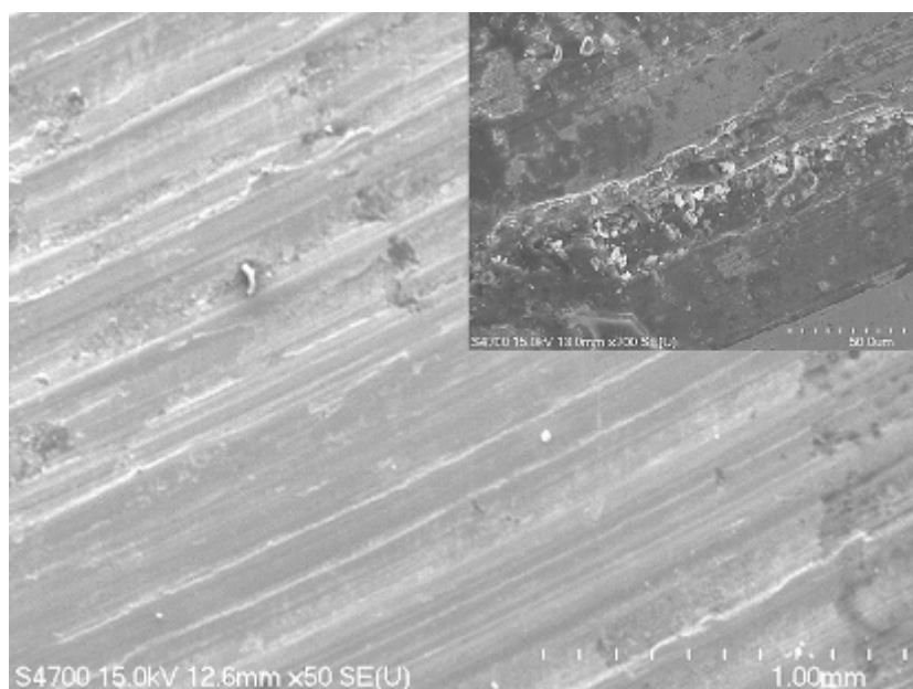
Fig.S5(a) The SEM image of worn surface of lower specimens in R68 oil without dUDD-PMMA lubricant additive.
