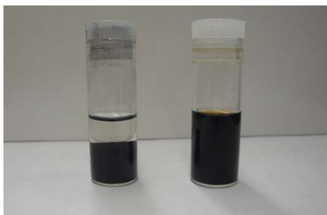
Fig. S4. Photograph of initial sol of PbTe (right) and the wet gel formed after addition of TNM (left).
