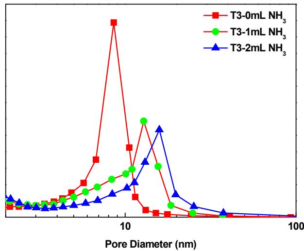
Figure S2. (Color online). Pore size distribution of three NH<sub>3</sub>-MS TiO<sub>2</sub> samples (pore size: 8.57 nm, 12.85 nm, 15.87 nm)
