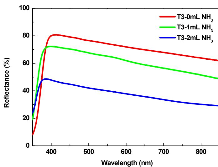
Figure S3. (Color online). Diffuse reflectance of three films made of the NH<sub>3</sub>-MS TiO<sub>2</sub> samples.
