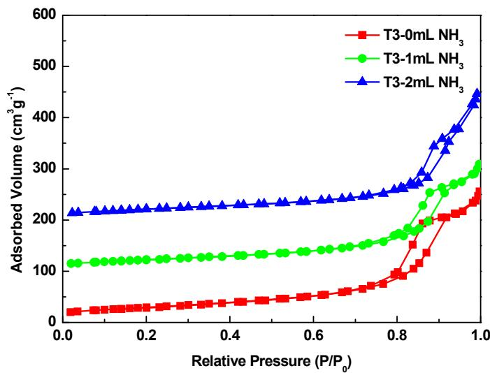
Figure S1. (Color online). Nitrogen sorption isotherms of the NH<sub>3</sub>-MS TiO<sub>2</sub> samples (T3-0 mL NH<sub>3</sub>, T3-1 mL NH<sub>3</sub>, T3-2 mL NH<sub>3</sub>). The isotherms of T3-1 mL and T3-2 mL are shifted by 100 and 200 cm<sup>3</sup> g<sup>-1</sup>, respectively, for the sake of clear presentation.
