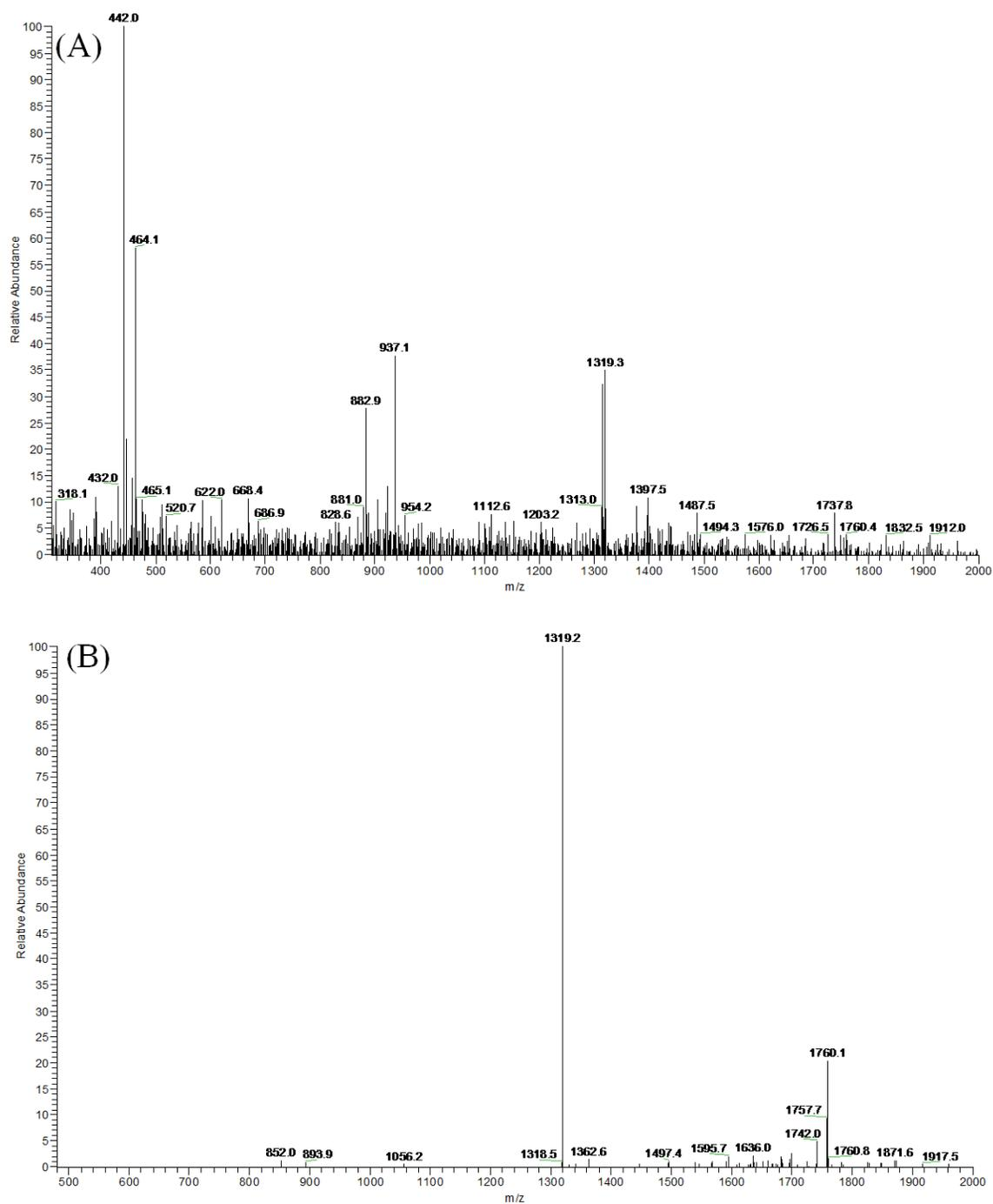
Figure S7. The MS spectra (A) and the MS/MS spectra (B) of  $\gamma$ -CD/FA inclusion complex.
