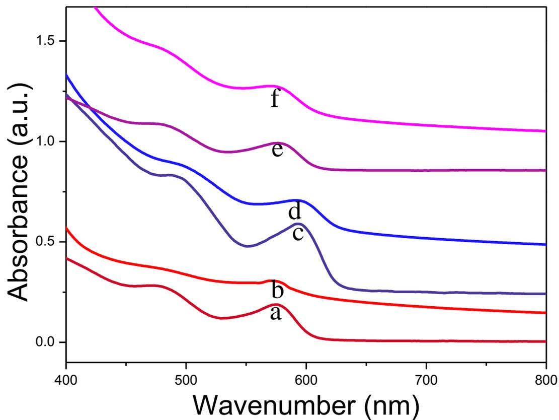
Figure S2. UV-vis spectra of TOPO-coated CdSe QDs (a), TOPO-coated CdSe/CdS QDs (c), TOPO-coated CdSe/ZnSe QDs (e) in chloroform, and  $\gamma$ -CD/FA-coated CdSe QDs (b),  $\gamma$ -CD/FA-coated CdSe/CdS QDs (d),  $\gamma$ -CD/FA-coated CdSe/ZnSe QDs (f) in PBS.
