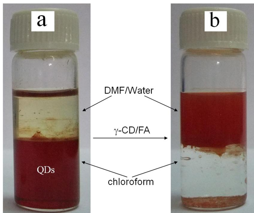
Figure S1. Photographs of the phase transfer experiments using quantum dots. The QDs in the chloroform phase (a) are transferred to the DMF/H<sub>2</sub>O phase (b) upon complexation of  $\gamma$ -CD/FA inclusion complex.
