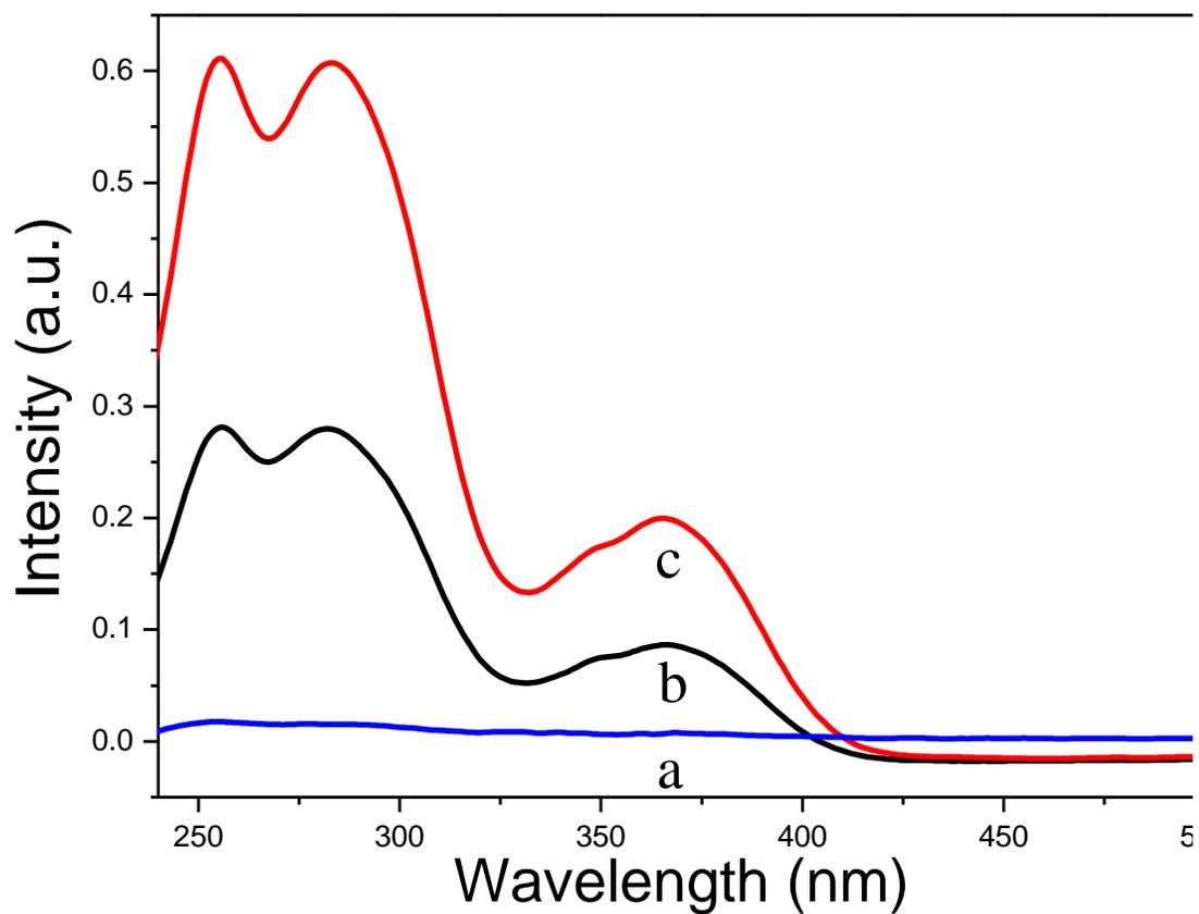
Figure S6. UV-vis spectra of  $\gamma$ -CD (a)  $\gamma$ -CD/FA inclusion complex (b) and FA (c) in 1.0 mM
