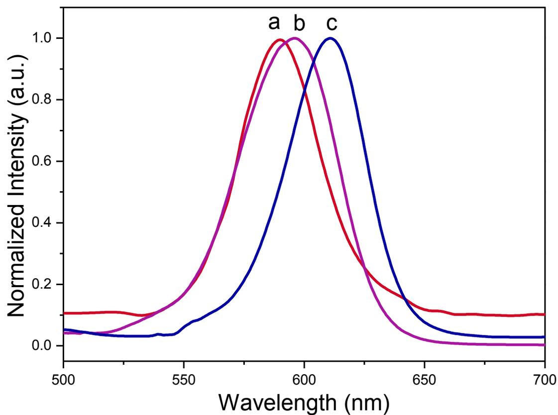
Figure S4. The luminescence spectra of three original QDs CdSe (a) CdSe/ZnSe (b) CdSe/CdS (c) in chloroform. Each sample was excited at wavelength with an absorbance value of 0.1.
