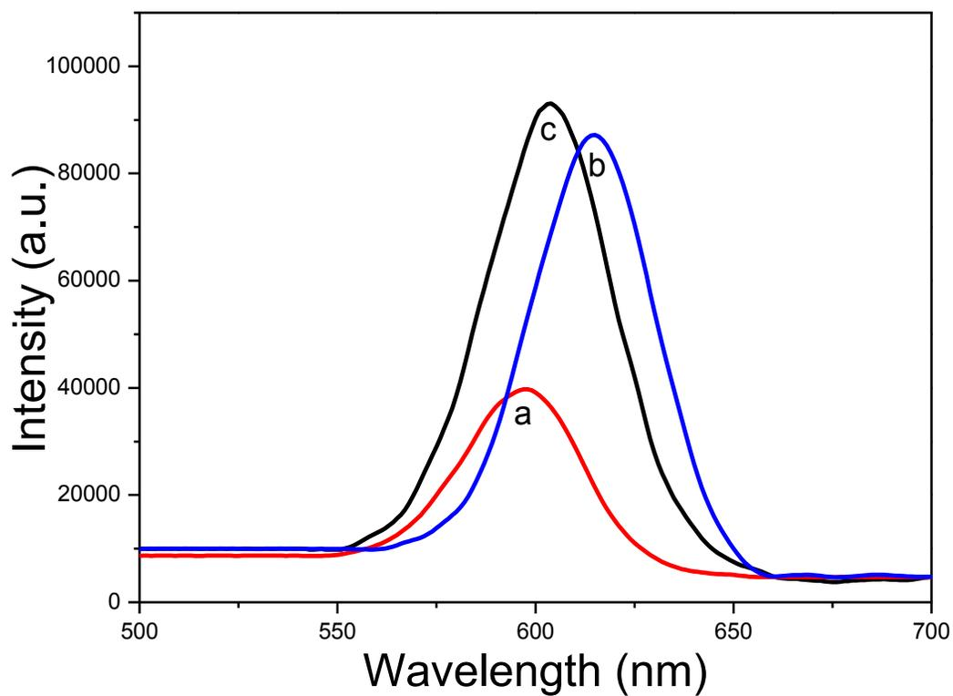
Figure S3. The luminescence spectra of  $\gamma$ -CD/FA-coated CdSe QDs (a),  $\gamma$ -CD/FA-coated CdSe/CdS QDs (b), and  $\gamma$ -CD/FA-coated CdSe/ZnSe QDs (c) in PBS. Each sample was excited at wavelength with an absorbance value of 0.1.
