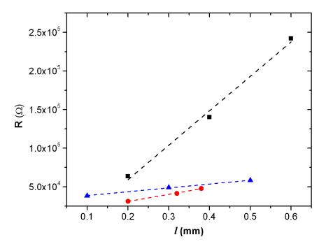
**Figure S1.** Resistance (R) of patterns with 3 ( $\blacksquare$ ), 5 ( $\bullet$ ), or 8 ( $\triangle$ ) bilayers versus distance between probe points (*l*) for 2-point conductivity measurements. Dashed lines were linearly regressed to the data.
