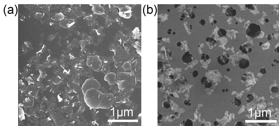
**Fig. S2** (a) SEM image, and (b) scanning helium ion microscope image, of the hBN sheets produced by ball milling in benzyl benzoate for 15 h and centrifugation at 376 g for 1 h.
