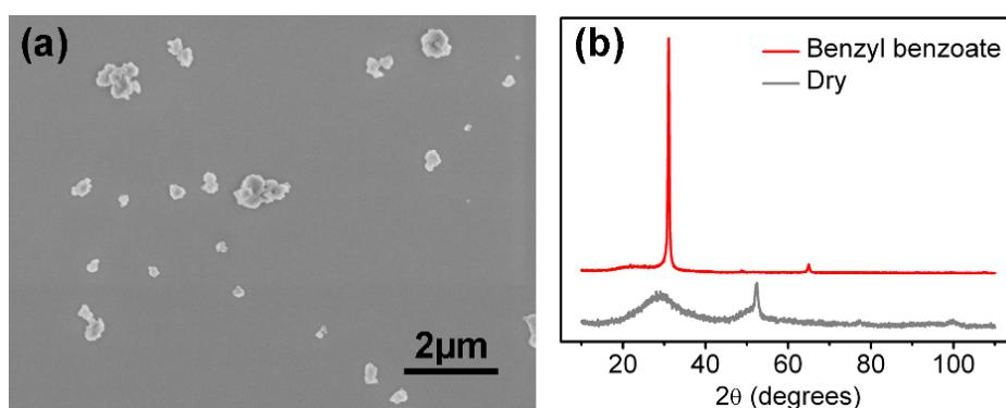
**Fig. S3** (a) SEM image showing the round-shaped BN particles after dry planetary milling for 15 h; (b) XRD spectra showing that the hBN milled in benzyl benzoate for 15 h still has a strong (002) diffraction peak, but the dry 15 h milled sample only shows a broad peak centred at 29.3° and a strong peak at 52.4° corresponding to steel contamination.
