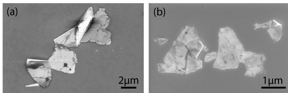
**Fig. S4** Typical SEM images of a cluster of BN sheets produced by (a) sonication in benzyl benzoate for 0.5 h and centrifuged at 376 g for 1 h; (b) sonication in benzyl benzoate for 0.5 h and centrifuged at 9391 g for 0.5 h.
