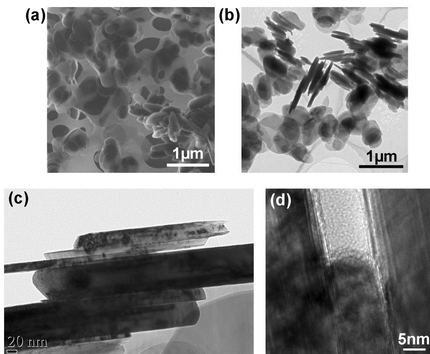
**Fig. S1** (a) Helium ion microscope image of the initial hBN particles; (b) low magnification TEM image of the hBN particles without milling; (c) edge view of a stack of hBN plates; (d) high magnification TEM image of the stack.
