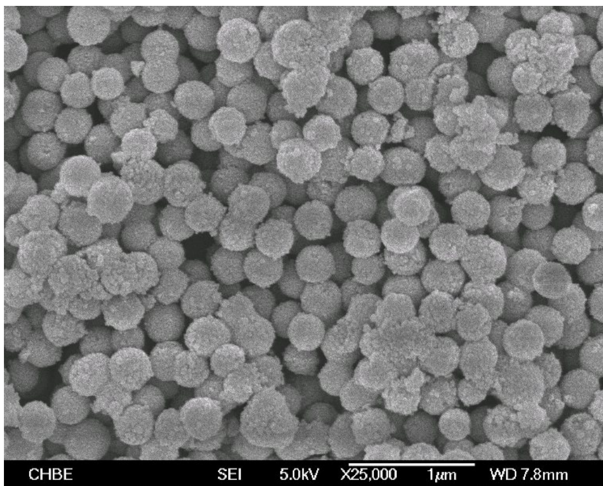
Fig. S3 SEM image for mesoporous F-TiO 2 spheres after being ultrasonicated in a water bath (400 W, 42 KHz) for 2 h.
