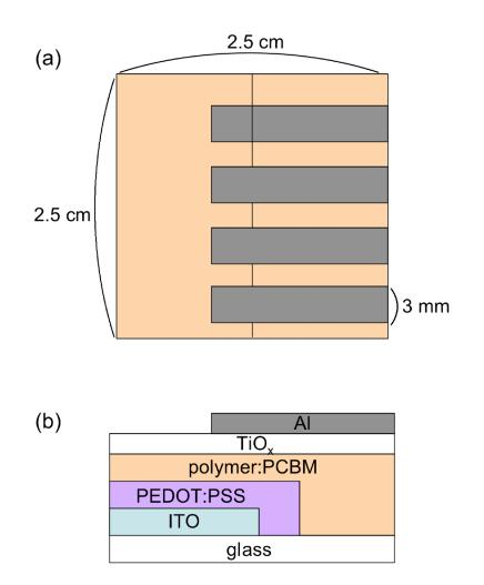
**Fig. S1** Schematic illustrations of (a) top and (b) side views of the ITO/PEDOT:PSS/polymer:PCBM/TiO<sub>x</sub>/Al device.
