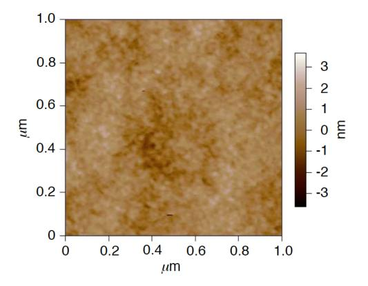
**Fig. S2** Tapping-mode atomic force micrograph of P3HT:PCBM film. The color scale represents the height topography, with bright and dark representing the highest and lowest features, respectively.
