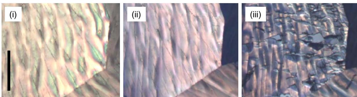
Fig. S6 Change of the DAE crystal film by excessive UV ( $\lambda=375$  nm) irradiation. (i) Uncolored film. (ii) Half-colored (surface) state. (iii) After excessive UV irradiation. Scale bar: 200  $\mu\text{m}$ .
