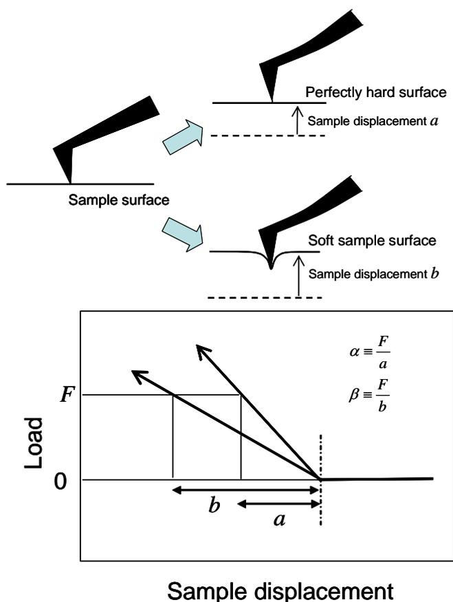
Fig. S3 Illustrations of FCs for obtaining the force per unit-indent-depth.
