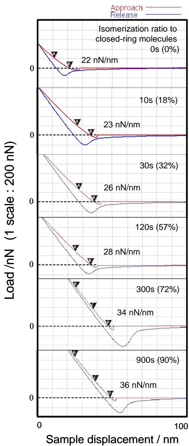
Fig. S2 Force curves of the amorphous DAE films with a thickness of 500 nm.
