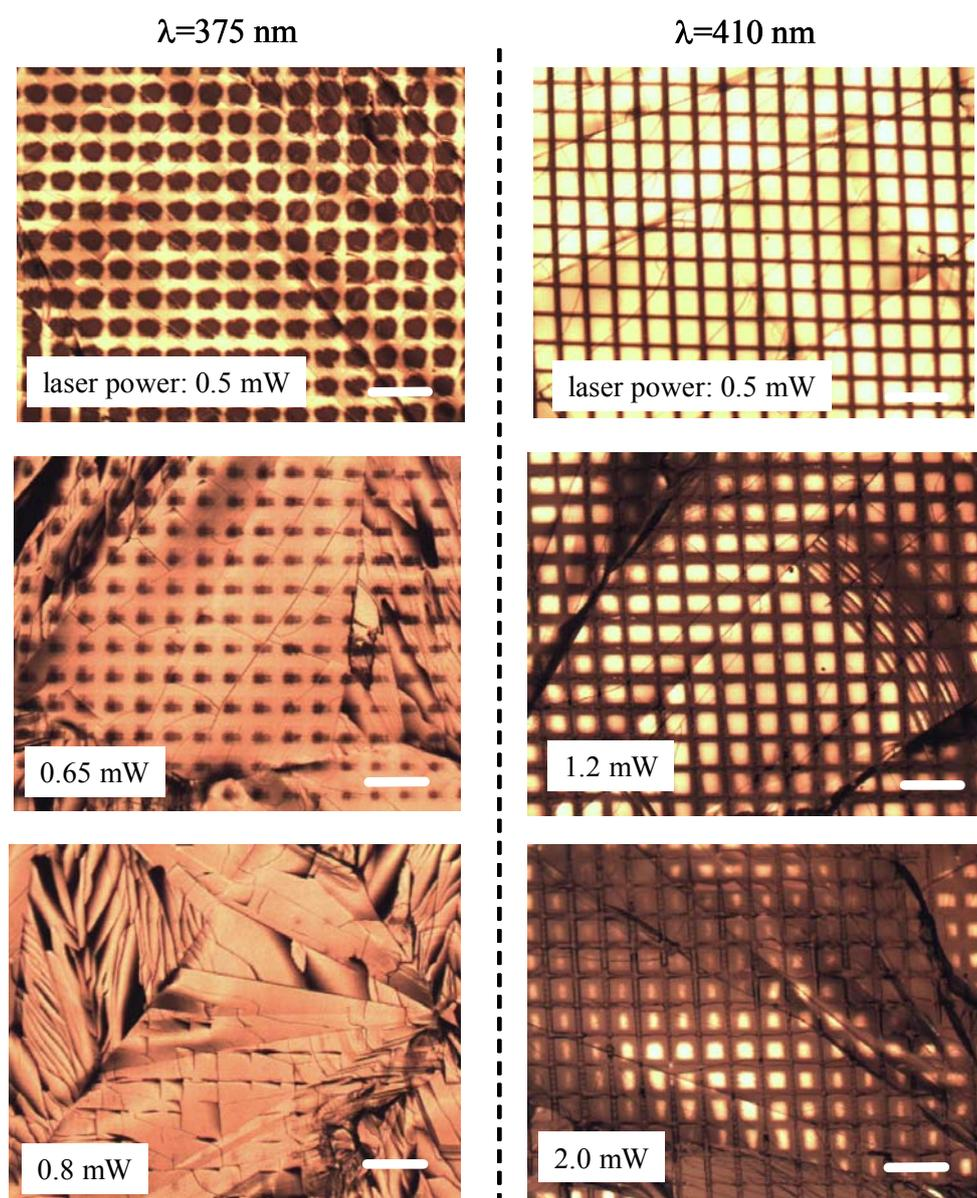
Fig. S5 Laser power dependence of Mg-deposition patterns on the DAE crystal surface. Laser scan speed: 2 mm/s. Bright areas show Mg deposited. Scale bar: 100  $\mu\text{m}$ .
