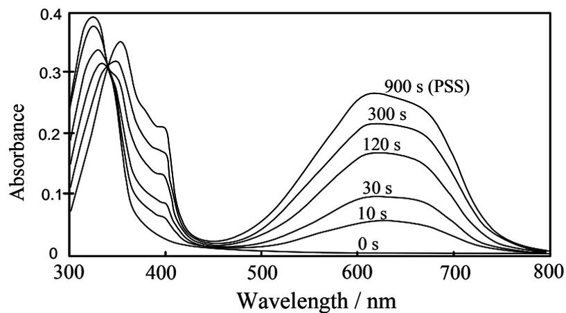
Fig. S1 Absorption spectra of the amorphous DAE films (thickness 50 nm) with various isomerization ratios. The samples were prepared by adjusting the irradiation of UV light ( $\lambda=365$  nm).
