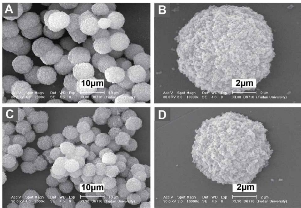
**Fig. S2** SEM images of  $\beta$ /UF-ZMSs (A-B) and  $\beta$ -ZMSs (C-D) prepared at  $n_{\text{HCl}} : W_{\text{nanozeolite}}$  of 4.5 mmol g<sup>-1</sup>.
