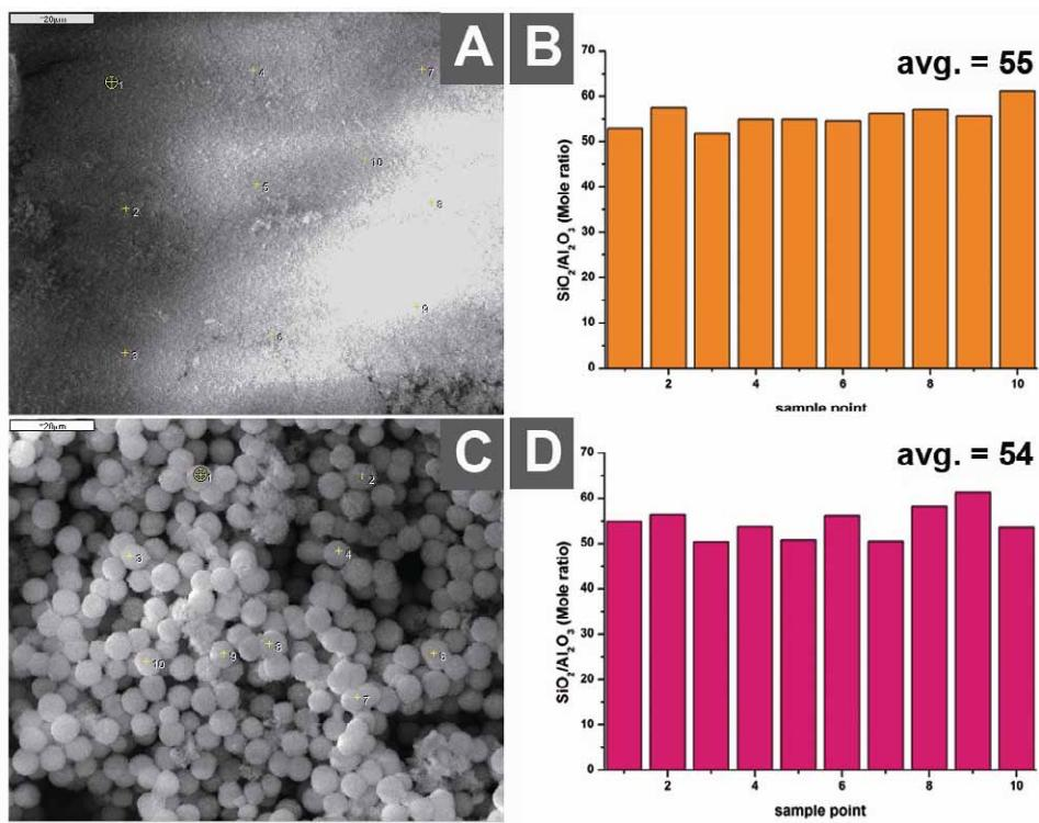
**Fig. S3** EDS analysis of nanozeolite  $\beta$  (A, B) and  $\beta$ -ZMSs (C, D) prepared at  $n_{\text{HCl}}:W_{\text{nanozeolite}}$  of 4.5 mmol g<sup>-1</sup>
