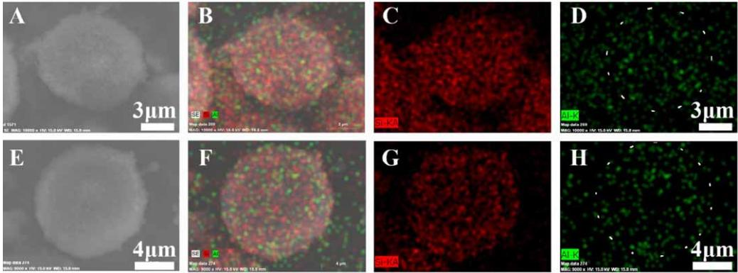
**Fig. S4** Element distribution of  $\beta$ /UF-ZMS as synthesized with adding HCl at  $n_{\text{HCl}}:W_{\text{nanozeolite}}$  of 4.5 mmol g $^{-1}$  (A-D, region II) and 23.25 mmol g $^{-1}$  (E-H, region III), respectively.
