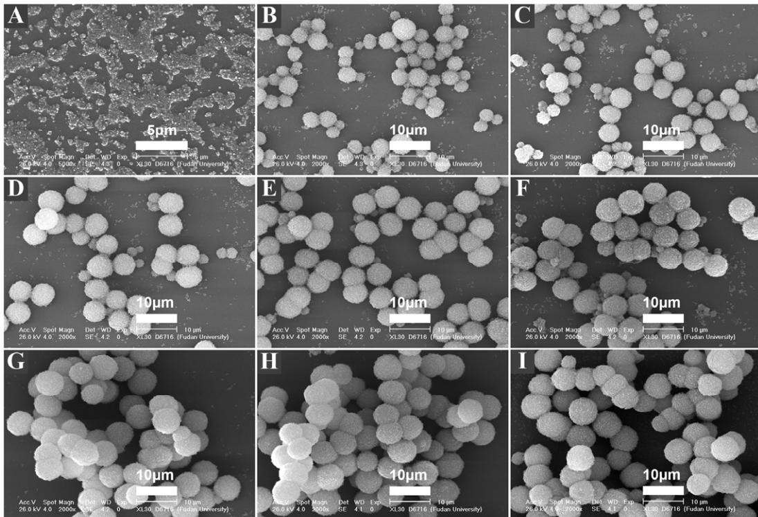
**Fig. S5** SEM images of  $\beta$ /UF-ZMSs directly collected from the reaction mixture at different time of 0 (A), 0.5 (B), 1 (C), 1.5 (D), 2 (E), 2.5 (F), 5 (G), 10 (H), 720 (I) min at  $n_{\text{HCl}}:W_{\text{nanozeolite}}$  of 12 mmol g $^{-1}$ .
