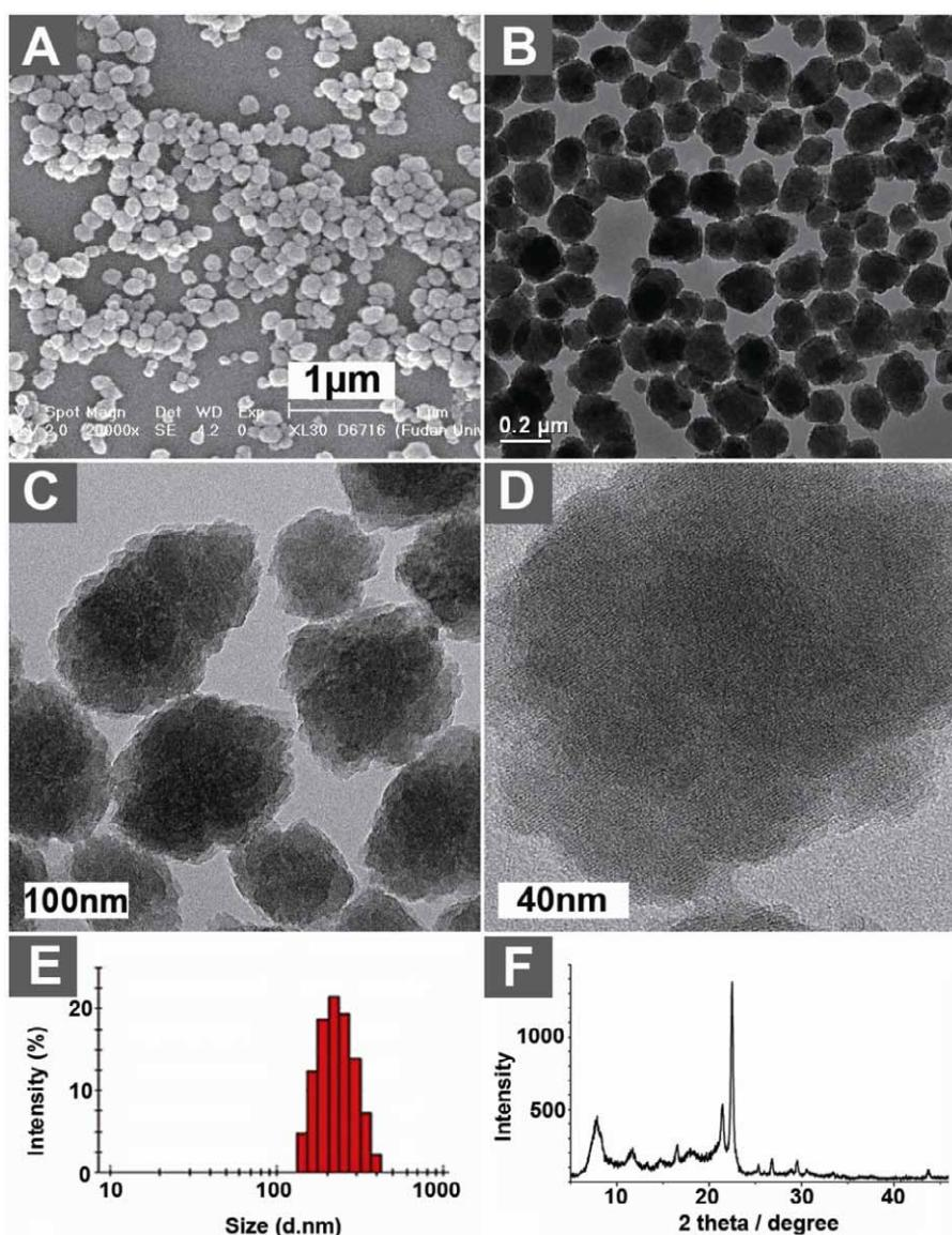
**Fig. S1** SEM image (A), TEM images (B, C and D), particle size distribution (E), XRD pattern (F) of nanozeolite  $\beta$ .
