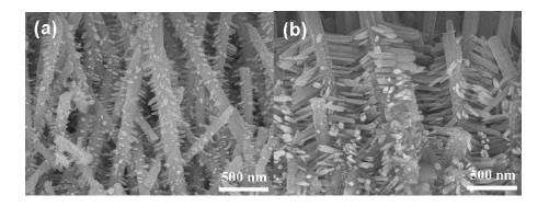
**Figure S1** Cross-sectional and high-magnification SEM images of (a) ZnO ND-30 and (b) ZnO ND-60 arrays.
