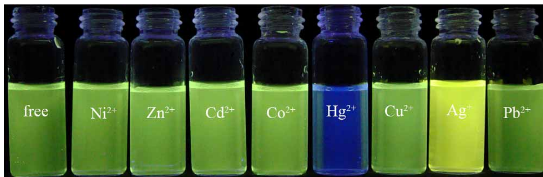
Fig. S9 Fluorescence images of 1 ( 1.0 \times 10^{-5} M) on addition of different metal ions in CH 3 CN–H 2 O (1:1, v/v) solution. Left to right: free metal ions, Ni 2+ ( 1.0 \times 10^{-4} M), Zn 2+ ( 1.0 \times 10^{-4} M), Cd 2+ ( 1.0 \times 10^{-4} M), Co 2+ ( 1.0 \times 10^{-4} M), Hg 2+ ( 2.0 \times 10^{-5} M), Cu 2+ ( 1.0 \times 10^{-4} M), Ag + ( 1.0 \times 10^{-4} M), Pb 2+ ( 1.0 \times 10^{-4} M).
