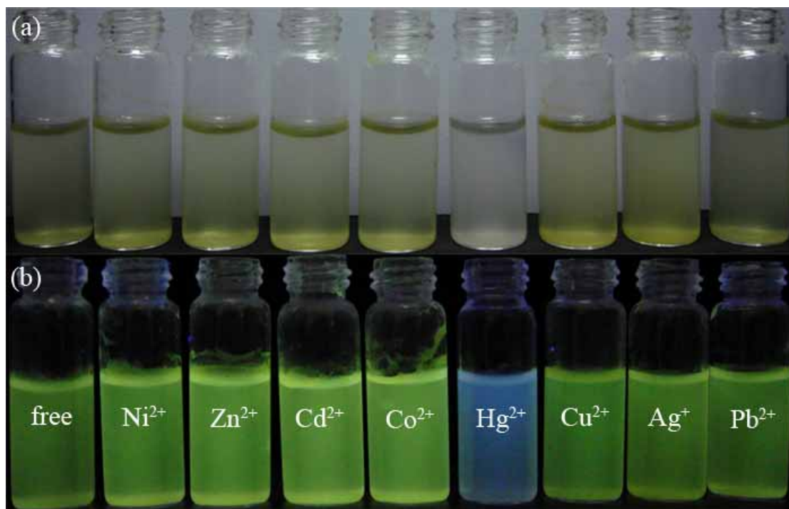
Fig. S14 (a) Color images and (b) fluorescence images of CH 3 CN–H 2 O (1:9, v/v) suspensions of MCM-3T (0.5 mg ml -1 ) on addition of different metal ions. Left to right: free metal ions, Ni 2+ , Zn 2+ , Cd 2+ , Co 2+ , Hg 2+ , Cu 2+ , Ag + , Pb 2+ .
