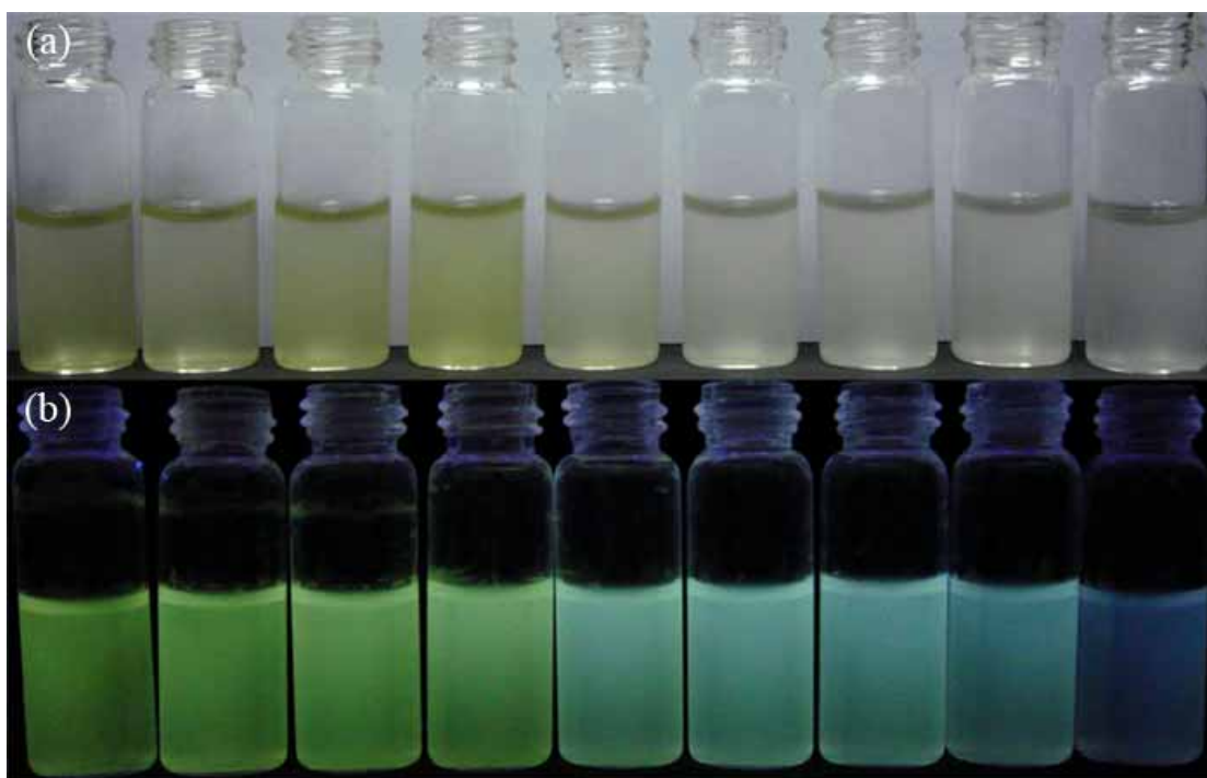
Fig. S13 Photographs of emission colors of MCM-3T ( 0.5 \text{ mg ml}^{-1} ) towards different concentrations of \text{Hg}^{2+} ( 0\text{--}4.0 \times 10^{-4} \text{ M} ) in \text{CH}_3\text{CN-H}_2\text{O} (1:9, v/v) solution under the radiation of (a) room light and (b) a UV lamp.
