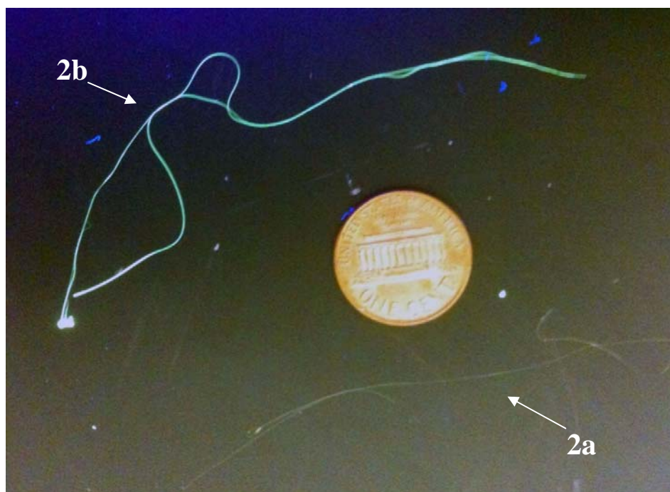
Figure S4. Photograph of melt-drawn fibers of compounds 2a and 2b irradiated with white and UV light.
