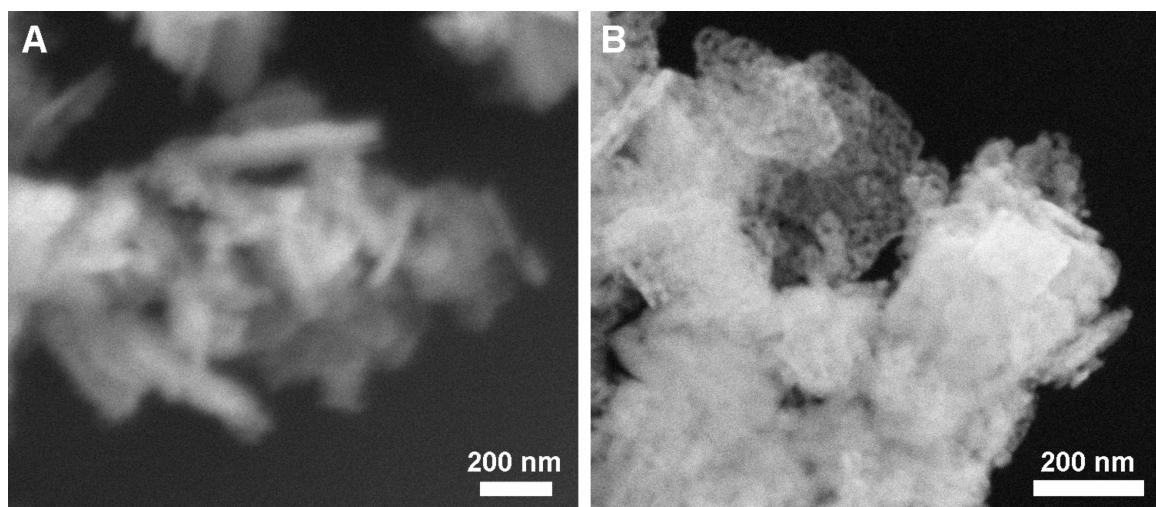
**Figure S6.** Scanning electron microscope images of MgO-325M after (A) preconditioning heat treatment and (B) an extended temperature exposure of 600 °C under nitrogen for 15 hours.
