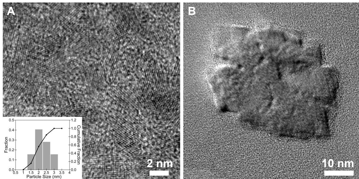
**Figure S1.** Transmission electron microscope images of as synthesized: (A) MgO-NP1, mean particle diameter is  $2.5 \pm 0.5$  nm. (B) MgO-NP2, with particle width ranging between 32 and 53 nm.
