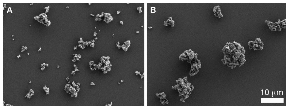
**Figure S5.** Scanning electron microscope images of preconditioned heat-treated (A) MgO-325M and (B) MgO-40M.
