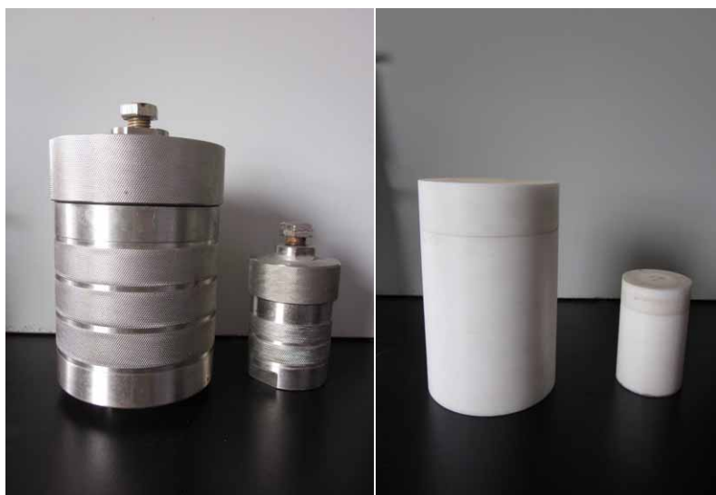
Fig. S2 Teflon-lined stainless steel autoclaves (500 mL and 50 mL) used to prepare NAC-capped CdTe: Zn 2+ QDs .(Left: stainless steel shell, Right: Teflon-lined inner liner)
