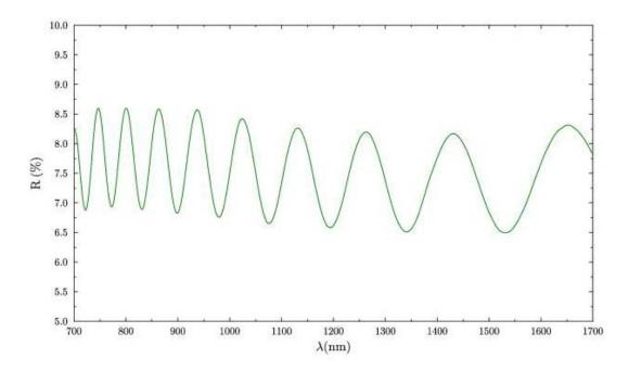
Reflectance spectrum of a polyurethane thin film, showing the interference pattern; the constant amplitude of the fringes in all the spectral range is a sign of good homogeneity and low surface roughness of the film.
