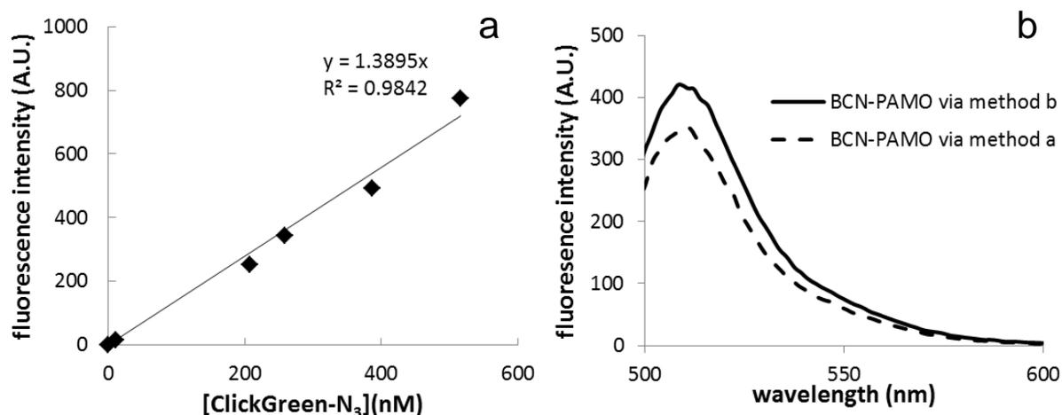
**Figure S2.** a) Calibration curve of ClickGreen-N<sub>3</sub> at  $\lambda_{\text{ex}} = 495 \text{ nm}$  in which the intensity at  $\lambda_{\text{em}} = 506.5 \text{ nm}$  is plotted against the concentration; b) emission spectra of ClickGreen-N<sub>3</sub> conjugated to BCN-functionalised PAMO.
