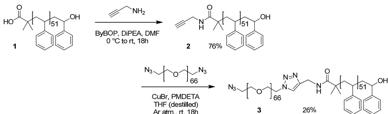
**Scheme 1.** Synthesis of PS<sub>52</sub>-*b*-PEG<sub>66</sub>-N<sub>3</sub> (**3**) through coupling of propargylamine to  $\alpha$ -carboxylic acid-polystyrene<sub>52</sub> **1**, followed by a Cu-catalysed 1,3-dipolar cycloaddition to N<sub>3</sub>-PEG<sub>66</sub>-N<sub>3</sub>.
