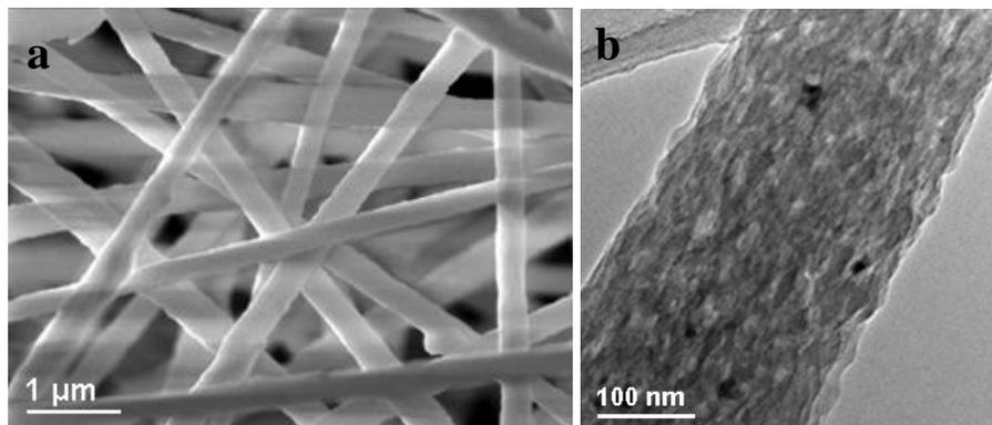
**Fig. S1** (a) FESEM and (b) TEM images of electrospun PAN/SnS hybrid nanofibers. Uniform nanofibers with diameter ranging from 300 to 400 nm were obtained through electrospinning. The length can reach up to tens of micrometer due to the continuity of electrospinning. The TEM image shows the homogeneous distribution of SnS in PAN nanofibers.
