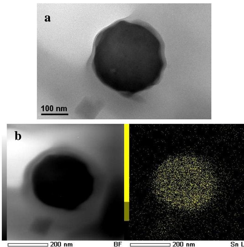
**Fig. S5** (a) Cross section TEM image and (b) corresponding STEM Sn mapping of carbonized PAN/SnS hybrid nanofibers. It is shown that element Sn distributes uniformly in carbon nanofiber, indicating that no diffusion occurs during carbonization. This is due to the high thermal stability and melting point of SnS.
