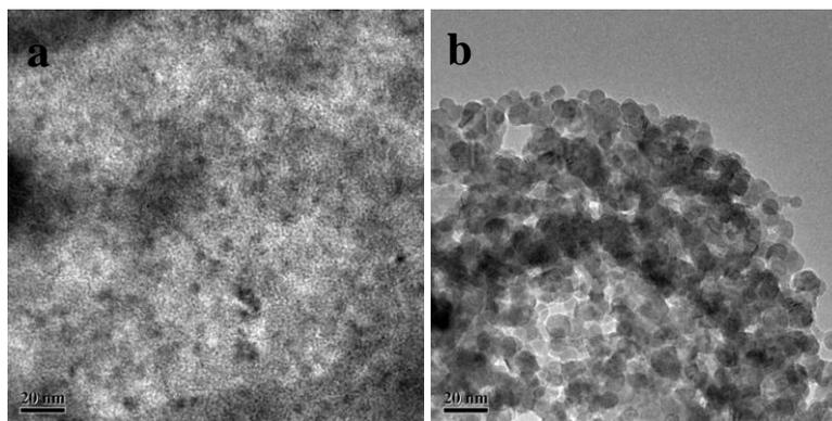
**Fig. S2** TEM images of (a) Sn(CH<sub>3</sub>COO)<sub>2</sub> and (b) SnSO<sub>4</sub> dispersed in PAN/DMF solution, indicating the size of tin salt nanoparticles is about 10 nm or less. The TEM samples were prepared by casting tin salt dispersion in PAN/DMF onto the copper grid.
