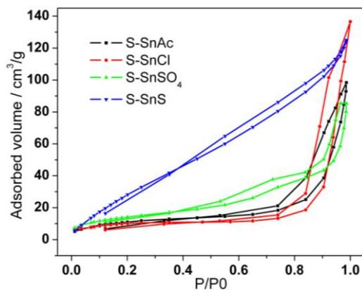
**Fig. S6**  $N_2$  adsorption/desorption isothermal profiles of  $SnO_2$  nanofibers/nanotubes from different precursors. Typical isothermal profiles are observed for  $SnO_2$  nanofibers/nanotubes derived from all precursors, in which SnS-derived  $SnO_2$  nanofibers clearly shows their higher surface area.
