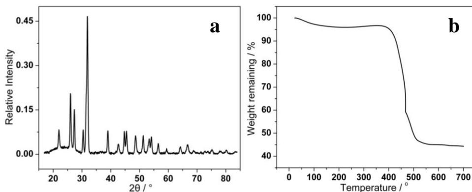
**Fig. S3** (a) XRD pattern of carbonized PAN/SnS hybrid nanofibers, indicating that SnS is not converted to  $\text{SnO}_2$  under the carbonization condition. (b) TGA curve of carbonized PAN/SnS hybrid nanofibers under the following condition: heated from room temperature to 700  $^\circ\text{C}$  at 10  $^\circ\text{C}/\text{min}$  in air, and kept at 700  $^\circ\text{C}$  for 10 min. The content of Sn-containing compound in carbonized hybrid nanofibers is measured to be around 45 wt%.
