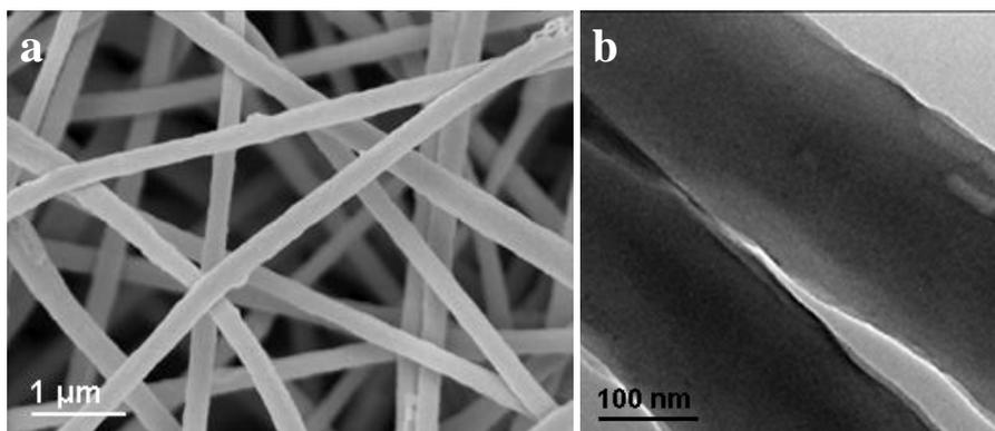
**Fig. S4** FESEM and TEM images of carbonized PAN/SnS hybrid nanofibers. The fibrous morphology is maintained after carbonization, while the diameter is reduced to 200-300 nm due to the formation of carbon upon cross linking and removal of N and H from PAN. The homogeneous morphology is also observed from TEM image, indicating the uniform distribution of Sn-containing mixture in carbon nanofibers.
