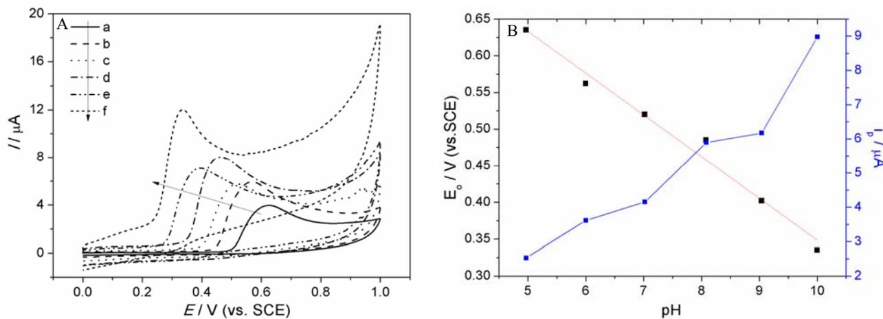
**Figure S6** (A) CV curves of 0.1 mM BPA at the proposed electrode modified with 20% of apatite under different pH: (a-f) 5, 6, 7, 8, 9 and 10. (B) The relationship between the oxidation potential and peak current, respectively. Other conditions are the same as Fig.S3.
