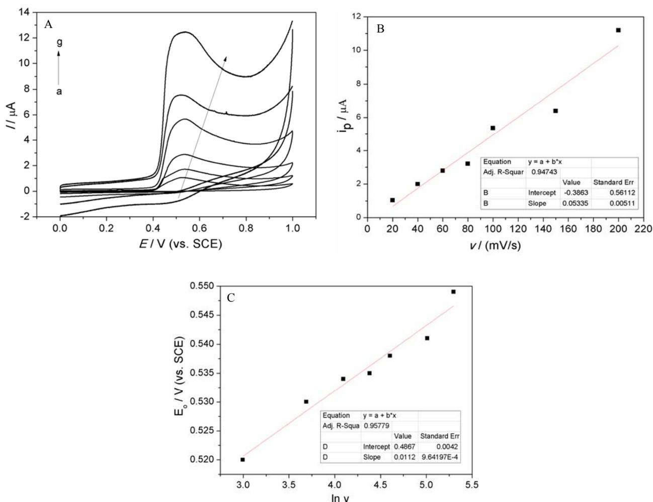
**Figure S7** (A) CV curves of 0.1 mM BPA at the proposed electrode modified with 20% of apatite with different scan rates: (a-g) 20, 40, 60, 80, 100, 150 and 200 mV/s. (B) Dependence of the oxidation peak current on the scan rate. (C) The relationship between the oxidation potential and  $\ln v$ . Other conditions are the same as Fig.S3.
