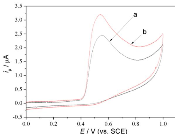
**Figure S4** CV behaviour of CMCPs modified by the products hydrothermally converted from (a) commercial  $\text{CaCO}_3$  and (b) egg-shell powder at 110 °C for 2 days. The measurement was performed in 0.2 M PBS containing 0.1 mM BPA with the scan rate of 100 mV/s.
