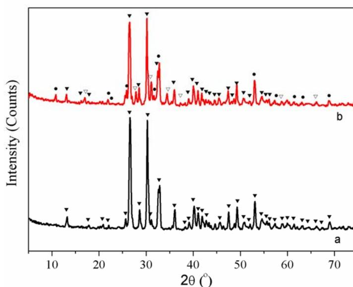
**Figure S3** XRD patterns of the products hydrothermally converted from (a) commercial CaCO<sub>3</sub> and (b) egg-shell powder at 110 °C for 2 days (●Ca<sub>10</sub>(PO<sub>4</sub>)<sub>6</sub>(OH)<sub>2</sub>
