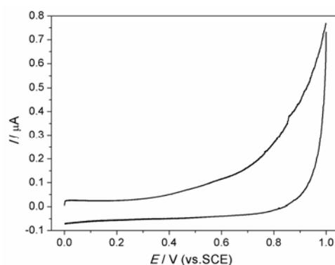
**Figure S2** Typical CV curve of electrode modified with 20% of 160°C-sample in pH 8 PBS.
