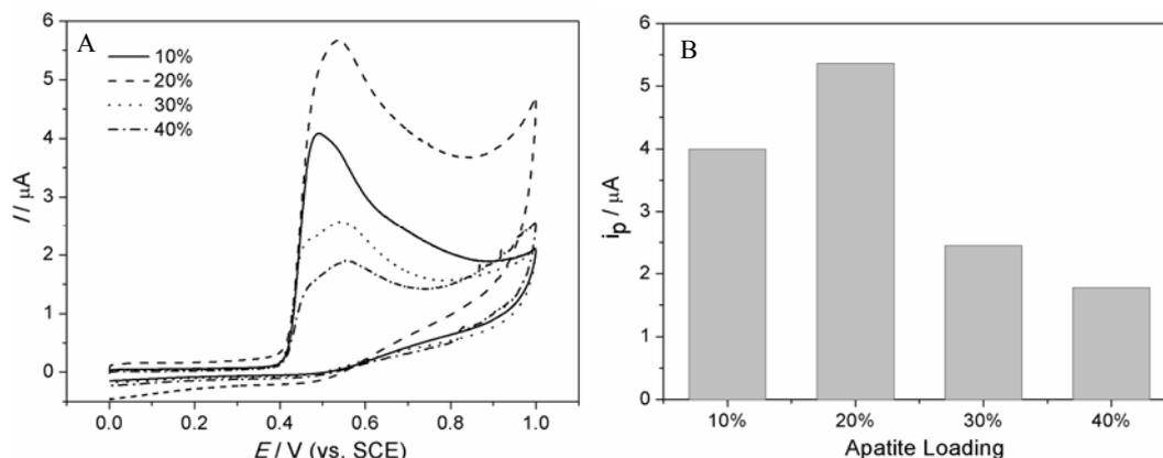
**Figure S5** (A) CV curves of 0.1 mM BPA at the proposed electrode modified with 10%, 20%, 30% and 40% of powders obtained from hydrothermal treated egg-shell at 160 °C for 2 days. (B) The relationship between the apatite loading and the peak current in (A).
